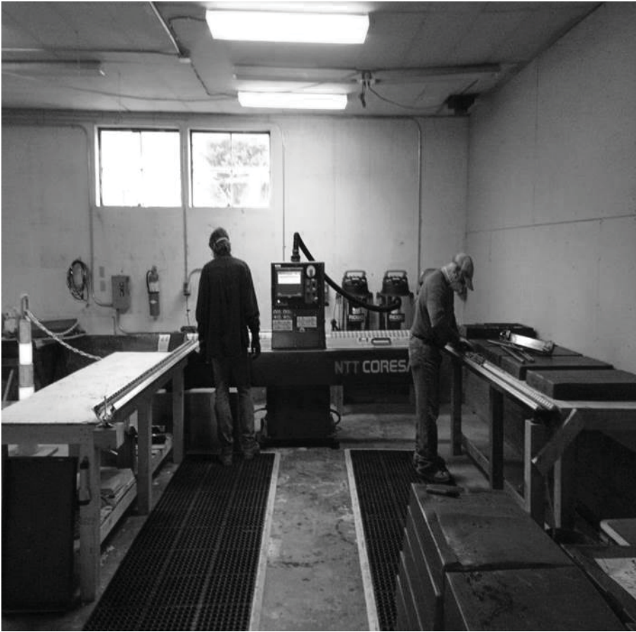
Figure 4. NTT Automated Core Saw (located against back wall) used on the Copper Cliff project
