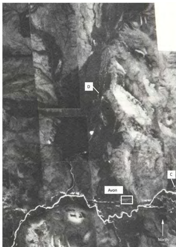
Figure 4. Thermal infrared imagery of the Warm Springs Creek that is tributary to Carpenter Creek near Avon, Site C is the largest spring on Warm Springs Creek; Site D shows bifurcation of Threemile Creek.
