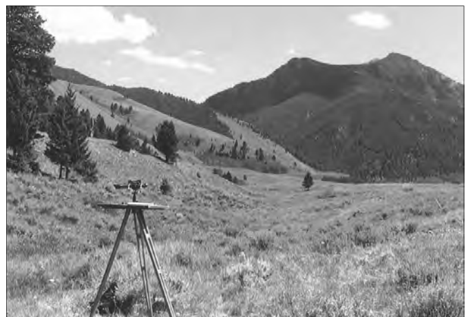
Figure 5. Alidade and plane table in south-eastward view along fault scarp with graben. Canyon of Sheep Creek is in background.
