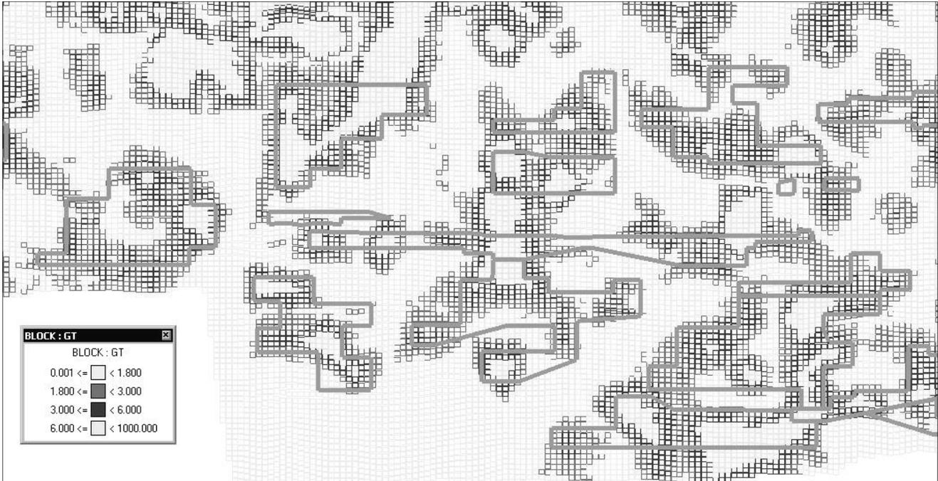
Figure 7. Grade –Thickness (opt-ft) contour of J-M Reef at Stillwater Mine (10'x 10' blocks)
