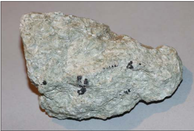
Figure 18. A fist-sized mass of intergrown radiating aggregates of prismatic tremolite crystals, Cable mine, Deer Lodge County, Montana.
