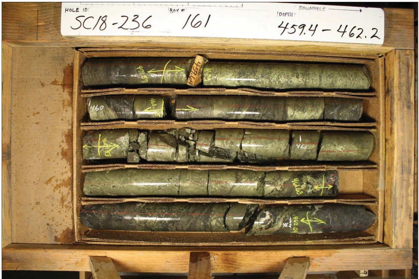
Figure 2. Drill core illustrating pyrite largely replaced by chalcopyrite from the Johnny Lee Lower zone.
