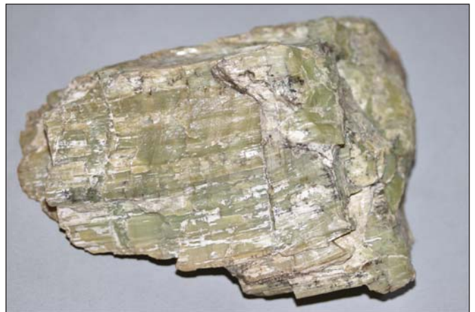
Figure 10. Fist-sized mass of lizardite showing slickenside texture from the Pomeroy mine, Deer Lodge County, Montana.
