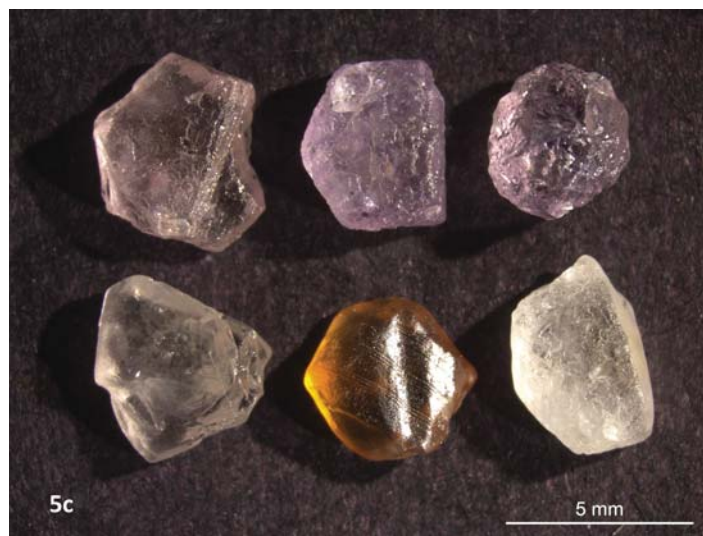
Figure 5. Rock Creek sapphires selected from jig concentrate: (a) incident white illumination; (b) LW UV illumination; (c) plain light illumination after heat treatment. Note the strong color change in the bottom center heat-treated stone.
