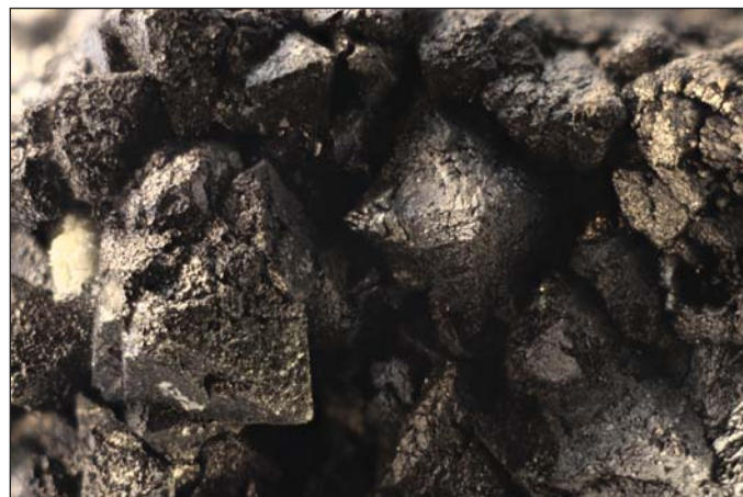
Figure 7. Large (2.5 to 3 cm) octahedral crystals of magnetite from the Pomeroy mine, Deer Lodge County, Montana.
