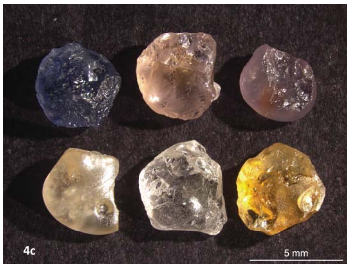
Figure 4. Rock Creek sapphires selected from jig concentrate: (a) incident white illumination, (b) LW UV illumination, (c) incident white illumination after heat treatment. The upper left and lower right stones yielded strong color change after heat treatment but did not display the strongest fluorescence.
