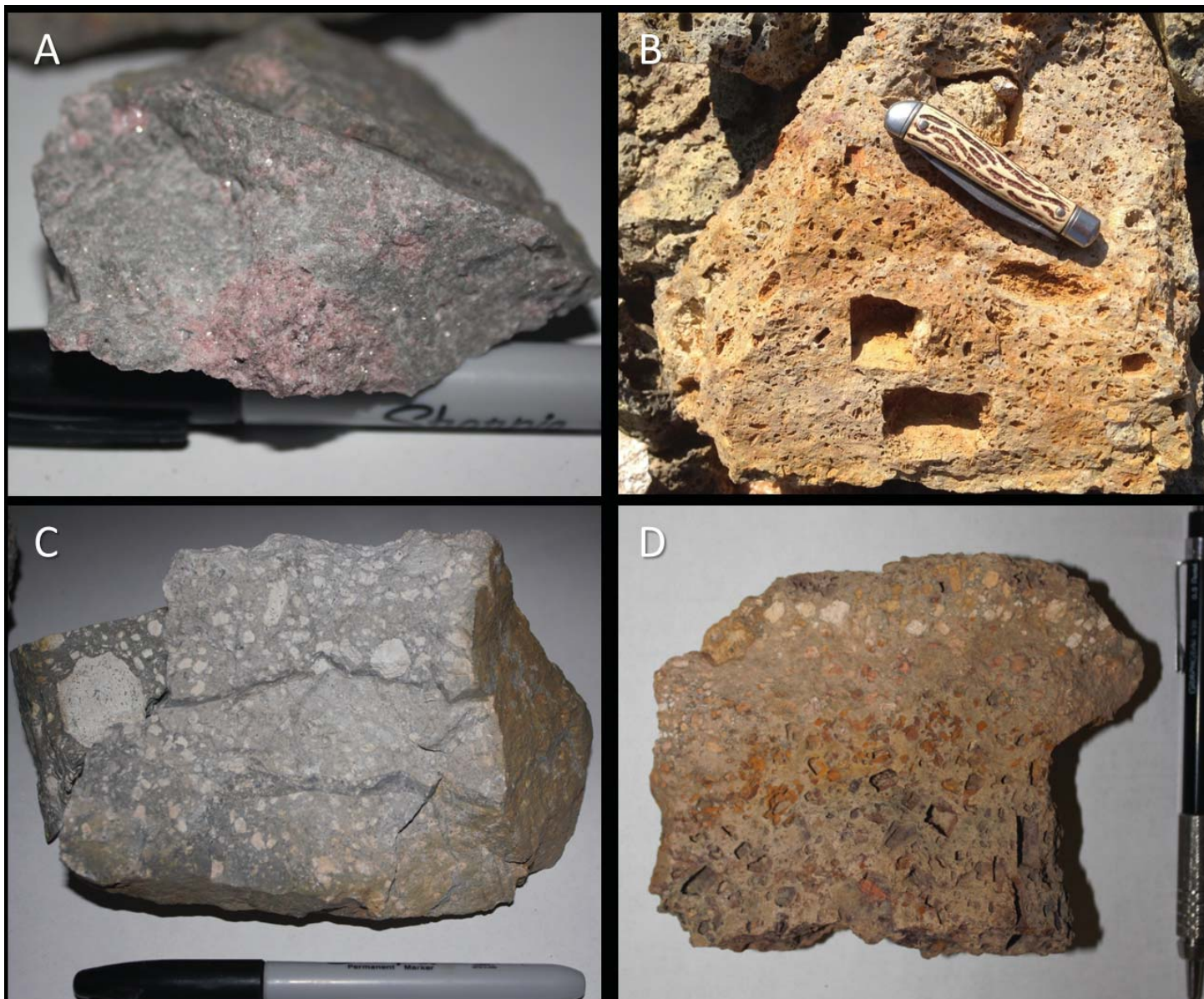
Figure 2. Advanced argillic alteration. (A) Pink, euhedral alunite. (B) Vuggy silica with sanidine feldspars completely dissolved. (C) Kaolinite (white) after feldspars. (D) Kaolinite, vuggy silica and Fe oxides.
