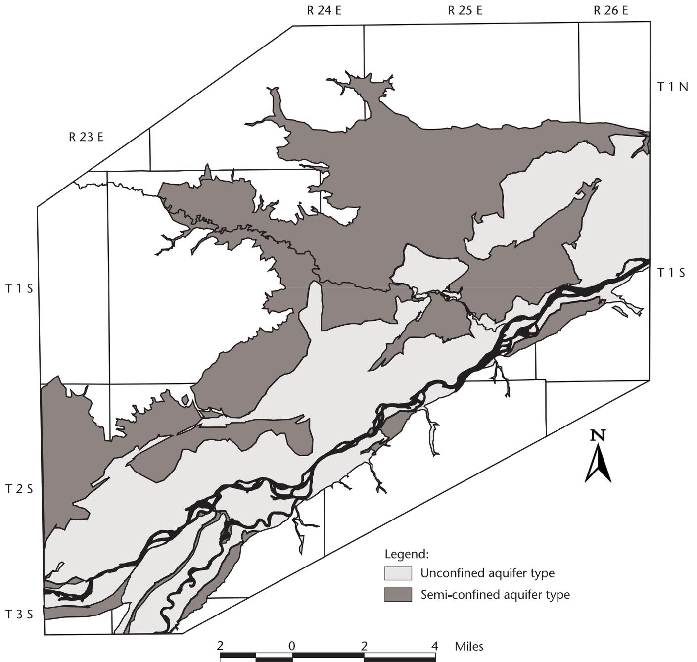
Figure 4. For most of the project area the fine-grained sediment layer acts to semi-confine the ground water.
