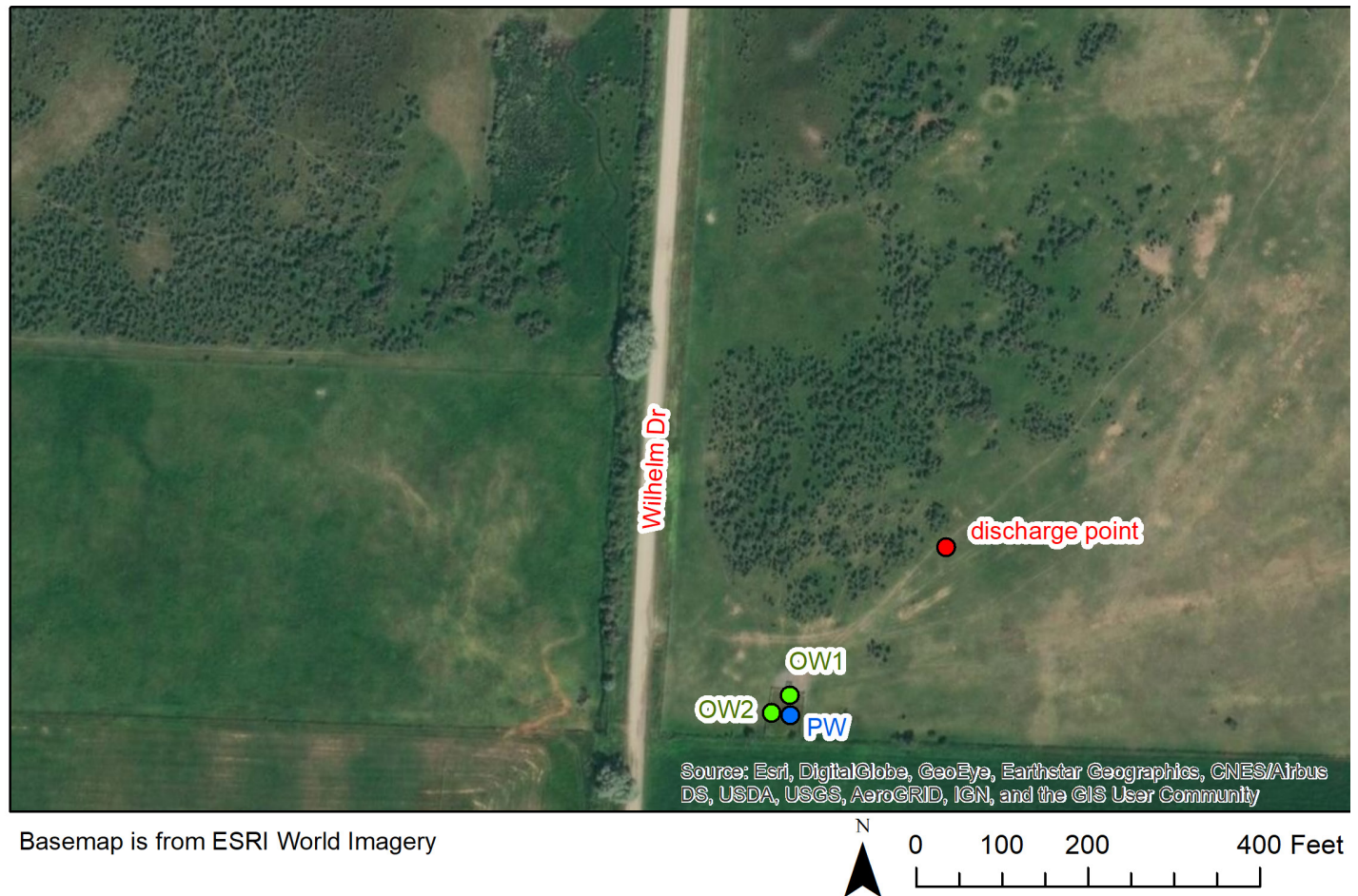
Figure 4-2. At the Hunt aquifer test site one pumping well and two observation wells were completed in the unconsolidated alluvium (table 3-1). During the tests, produced water was discharged approximately 300 ft northeast of the pumping well.
