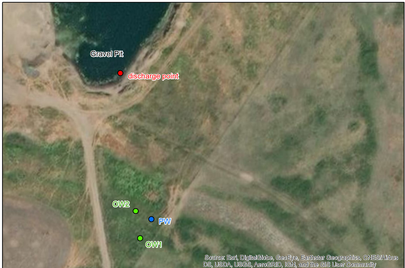
Figure 5-2. The Lazy TP Floodplain test site had a pumping well (PW) and two observation wells installed in the Renova Formation. During the tests, water was discharged into the unused flooded gravel pit approximately 225 ft north of the pumping well.
