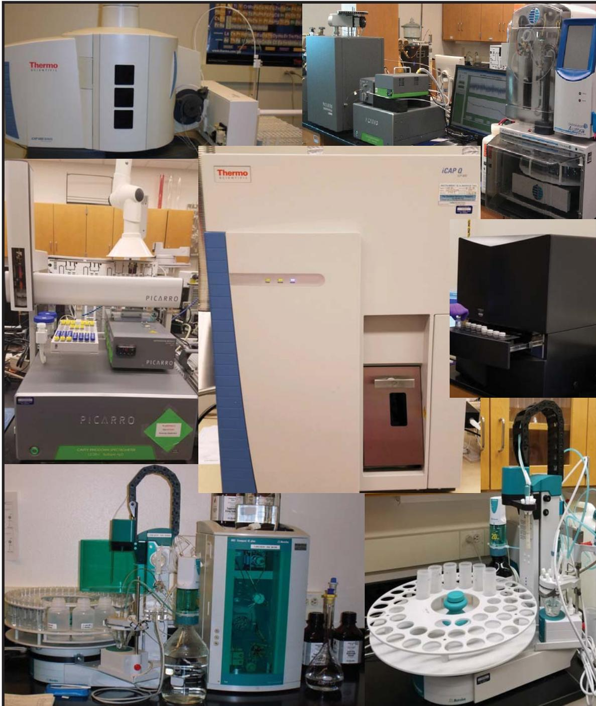
*Cover photo: Instruments in the MBMG Analytical Laboratory in 2020. Top row: Thermo iCAP 6000 ICP-OES, Picarro G2131-I  $\delta^{13}\text{C}$  High-Precision Isotopic carbon dioxide ( $\text{CO}_2$ ) analyzer. Middle row: Picarro L2130-I Isotopic Water Analyzer, Thermo iCAP Q ICP-MS, and HIDEX 300SL Auto TDCR Radon Analyzer. Bottom row: Metrohm 882 IC Plus Anion Chromatograph, Metrohm 855 Robotic Titrator. Photos by Jacqueline Timmer.*
