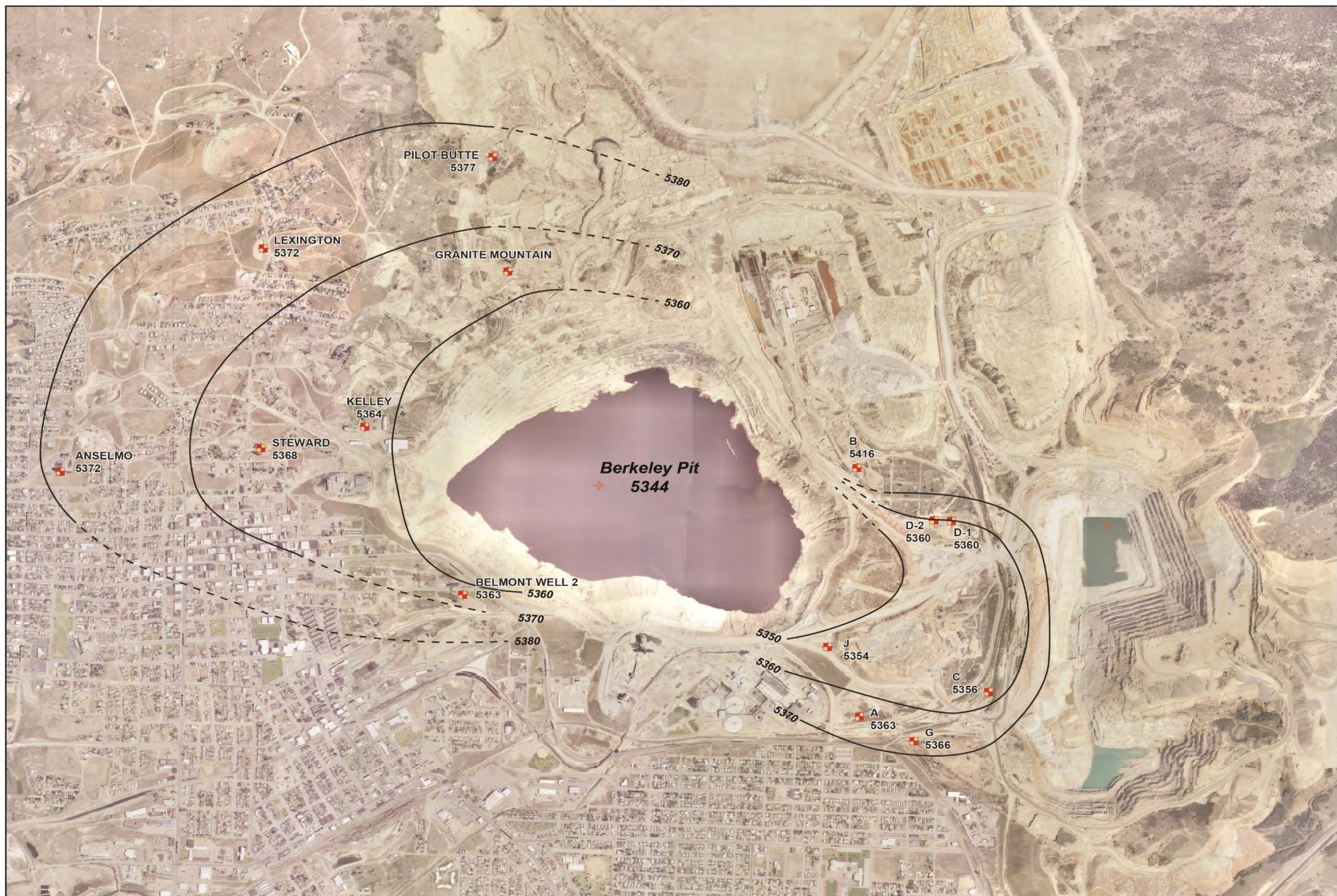
Figure 3-15. Potentiometric map for the East Camp bedrock aquifer, December 2018 (contour interval is 10 ft).
