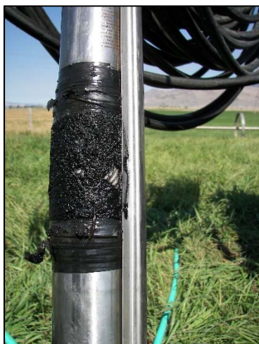
Figure 2. Clogged well screen.
