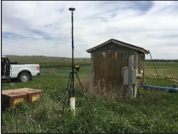
Figure 12. MBMG-239610 survey and steel protective casing.
