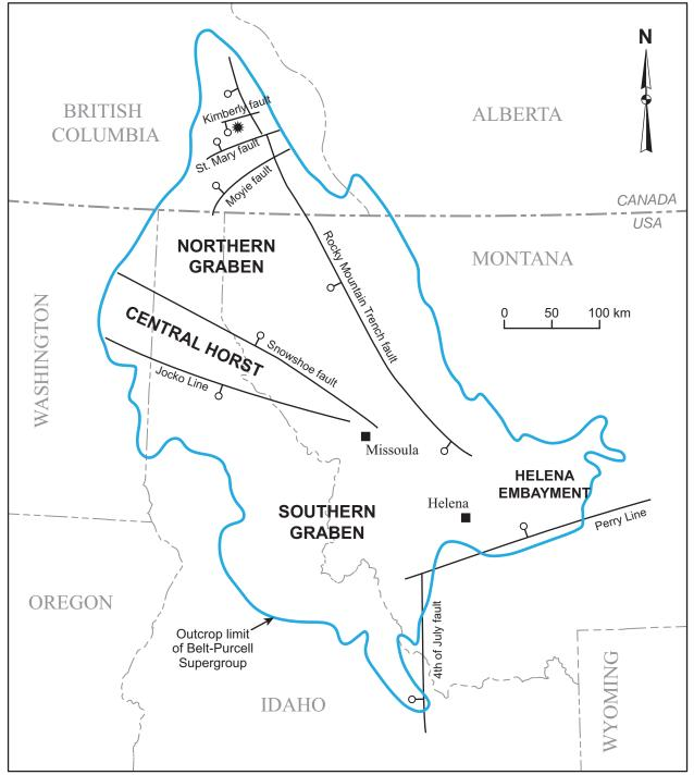
Figure 18. Lydon's interpretation of synsedimentary growth faults in the Belt Basin is based on thicknesses of the lower Belt in the northern part of the Belt Basin and on Sears' (2007a) unrestored syndepositional faults (see fig. 16, this paper). Star marks location of the Sullivan deposit along the Kimberly fault. Compiled from Lydon (2005, 2007) and Lydon and van Breemen (2013).
