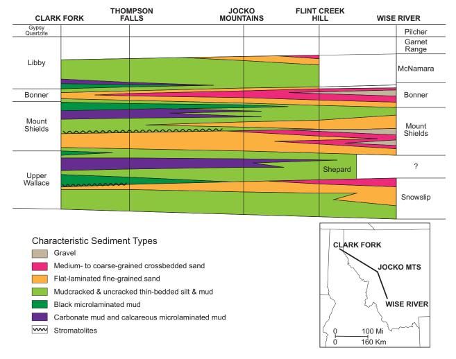
Figure 10. North–south fence diagram of Missoula Group lithologies shows how the sand wedges pinch out basinward and illustrates facies changes that occurred along the alluvial aprons that originated to the south (right). Note that the microlaminated mud is interpreted to represent deposition on very shallow mudflats. Modified from Winston, 1986a.
