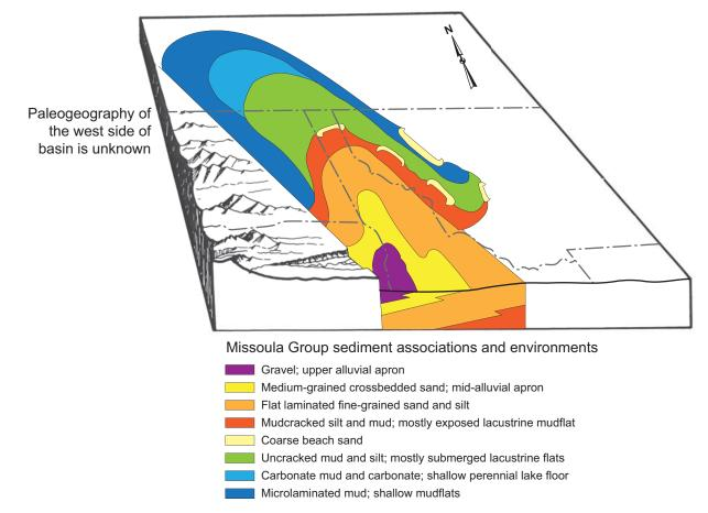
Figure 11. Block diagram shows facies associations during deposition of the Missoula Group. Sand and gravel facies alternately prograded and retreated, bordered by exposed mudflats of silt and desiccation-cracked mud that passes seaward to uncracked silt and mud and carbonate-bearing mud. Note that microlaminated mud was deposited on shallow mudflats near the shores of the Belt Sea. Modified from Winston, 1986a.
