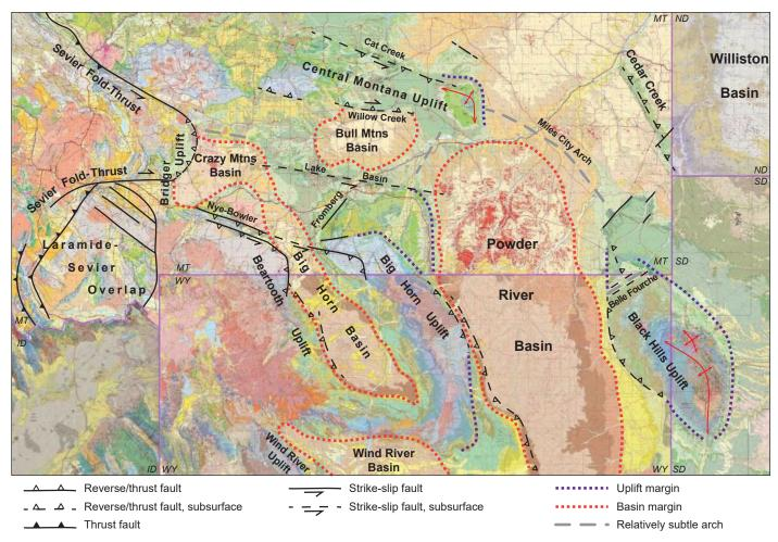
Figure 2. Regional Laramide uplifts, basins, linear features, and other structures. State geologic map base from U.S. Geological Survey National Geologic Map Database.
