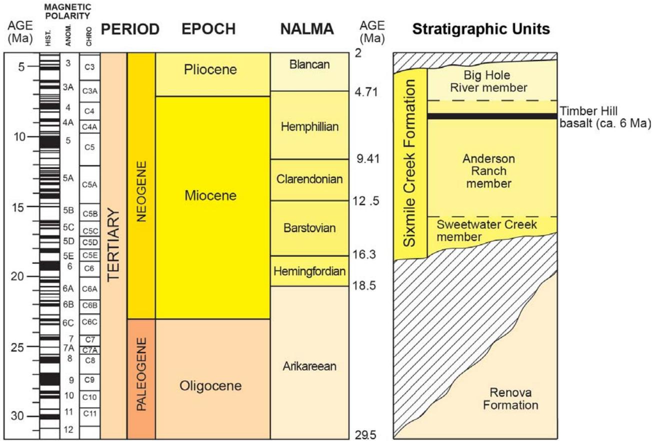
Figure 3. Generalized stratigraphy of the Sixmile Creek Formation (modified from Fritz and Sears, 1993). The Timber Hill basalt occurs only in the Ruby Graben in southwest Montana, and all members are not recognizable in every area where the Sixmile Creek Formation is mapped in Montana. Land mammal ages from Woodburn and Swisher (1995).
