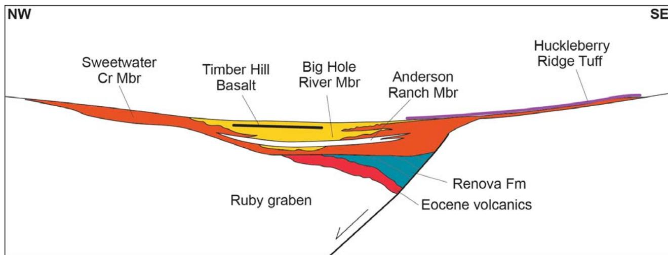
Figure 13. Schematic cross section of the middle Miocene Ruby graben in southwest Montana showing the Hemingfordian unconformity between the Renova Formation and older rocks and the overlying Sixmile Creek Formation. Modified from Sears and others, 2009.
