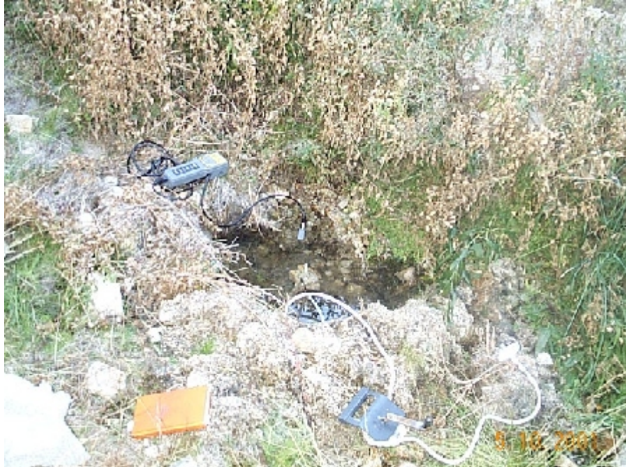
Figure 6a. The discharge sample (RUNS10M) was collected from a small pool near the adit.
