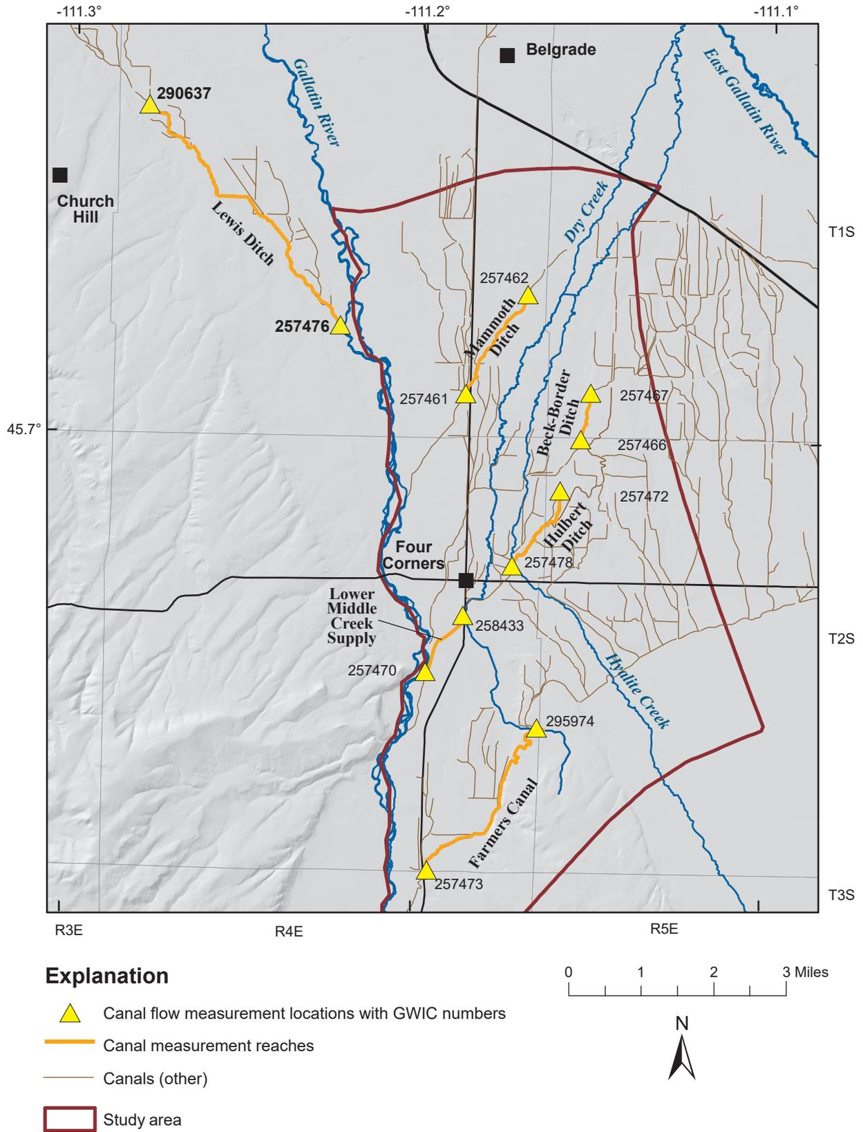
Figure 9. Flow measurements were made on six canals to estimate leakage rates.
