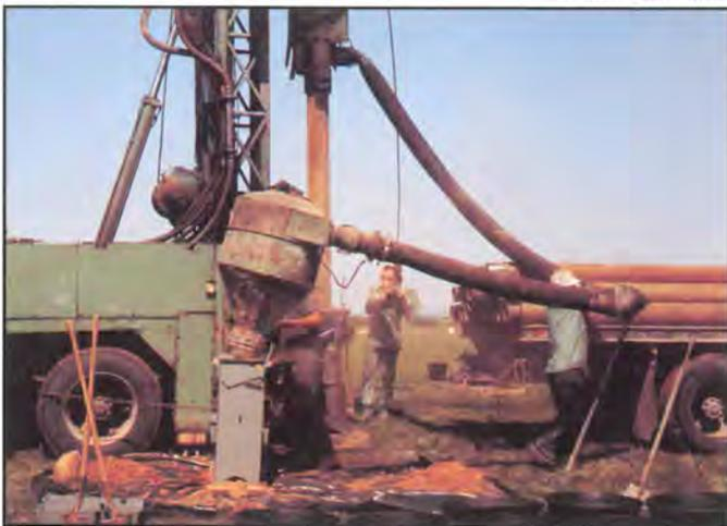
Drilling is expensive. Deposits containing coarse gold may not be assessed accurately by this method as the recovered sample is usually quite small. Most near-source placer deposits have spotty values and must be analyzed using large samples on close intervals. Deposits that are distant from the source may be more evenly dispersed, have smaller sized gold particles, and be more easily evaluated using drilling techniques.
