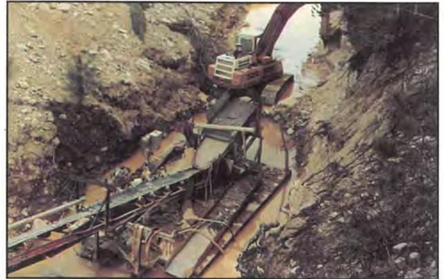
Floating wash plant used in a mobile operation.
