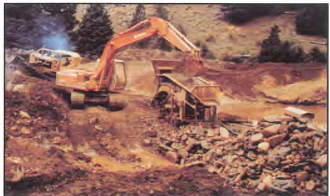
Follow drilling or trenching with a small (10 - 100 yd<sup>3</sup>) bulk sampling program to verify the results of the testing program. This will allow for testing the deposit, mining methods, and recovery equipment. A typical sample usually does not exceed a few hundred cubic yards of gravel.
