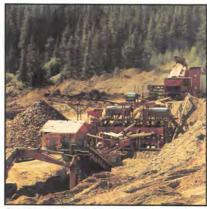
Overburden/spoils, silt, topsoil, sand and gravel piles should never be placed closer than 15 feet from the drainage. Use berms, silt fences, and/or straw bales to eliminate sedimentation from storm runoff.
