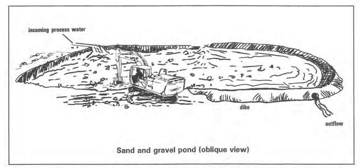
Sand and gravel ponds provide temporary storage of processed sand and gravel before use for reclamation at stationary placer operations.
