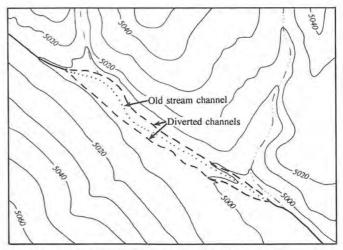
Diversion ditches (for surface water) should collect water from feeder drainages both upstream from the work area and from side drainages, and should deliver water to the stream below the operation. If necessary, a small ditch along either side of a wider valley can be very effective in controlling excess surface water.
