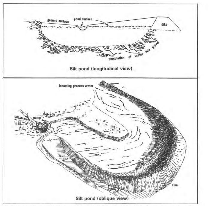
Construct settling ponds in undisturbed gravel rather than the fill material of the dike. The excavated material will form the dike, providing inexpensive material handling costs for pond reclamation and construction. Percolation from the pond into gravels removes surplus water and eliminates sedimentation to surface water.
