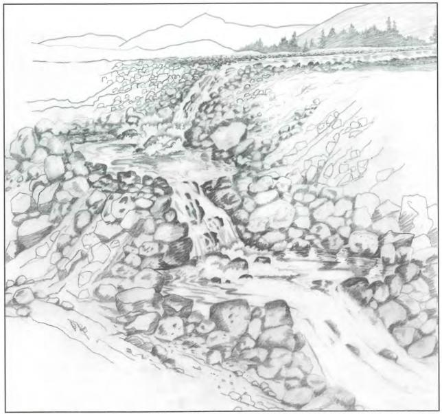
In steep mountainous environments, short stretches of heavily armored channel may be used to cascade the water to a lower elevation with minimal erosion and siltation. A small pool or silt trap at the bottom of each run will settle out fines and reduce the velocity in the channel.
