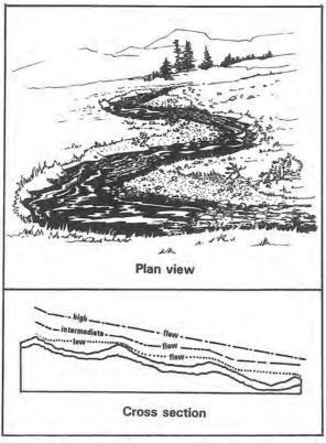
Views of channelbed elevation showing repeating pool riffle sequences (Inter-Fluve, Inc., 1991).
