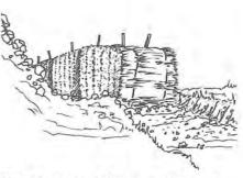
Weed-free straw bales may be used temporarily in place of berms for sediment control in the active mine area.
