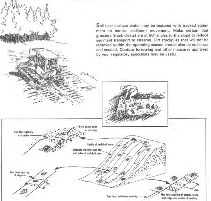
Erosion control blankets made of jute, straw, or plastic netting placed over seed and mulch will protect recently reclaimed highly erosive soils on steep slopes until vegetation is established.
