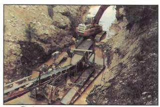
Floating wash plant used in a mobile operation.
