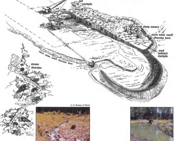
Divert surface waters and runoff from undisturbed land around the site.
