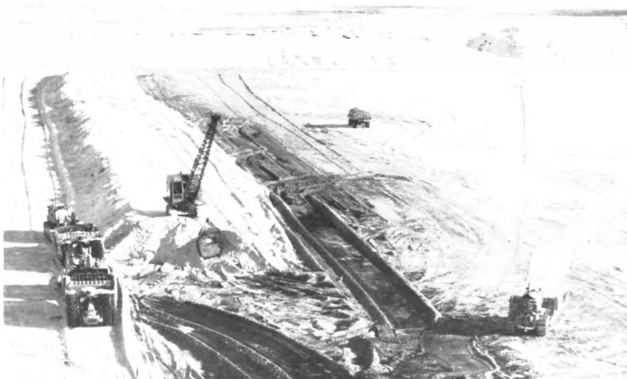
Figure 2-7.—Direct mining of the permanent crystalline bed in the shallow basin at the south end of Ingebright Lake.
