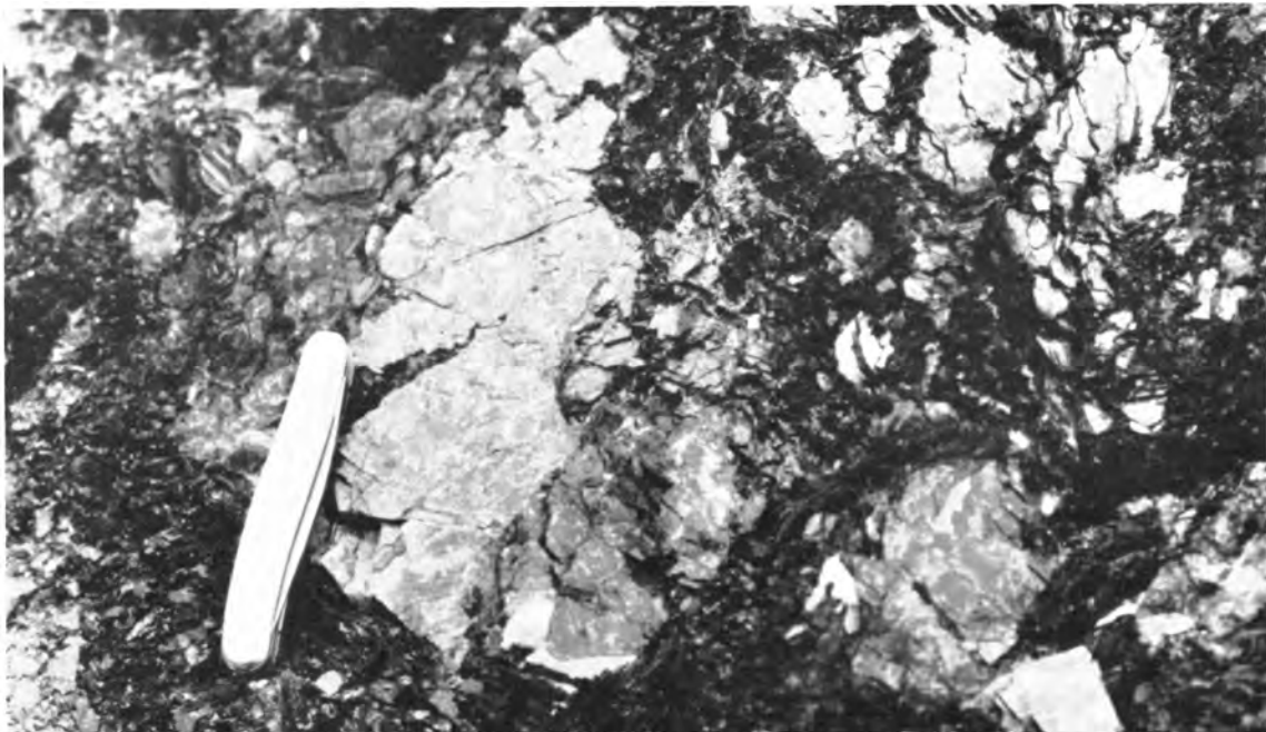
Figure 11-9.—Vermiculite and biotite in the biotite-pyroxenite pluton, Rainy Creek mine, Libby, Montana. Largest crystal is biotite; about three-fourths of rest of face is vermiculite. (Knife is 3¼ in. long.)
