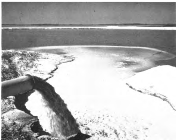
Figure 2-4.—Pumping brine from Chaplin Lake into reservoir ponds.
