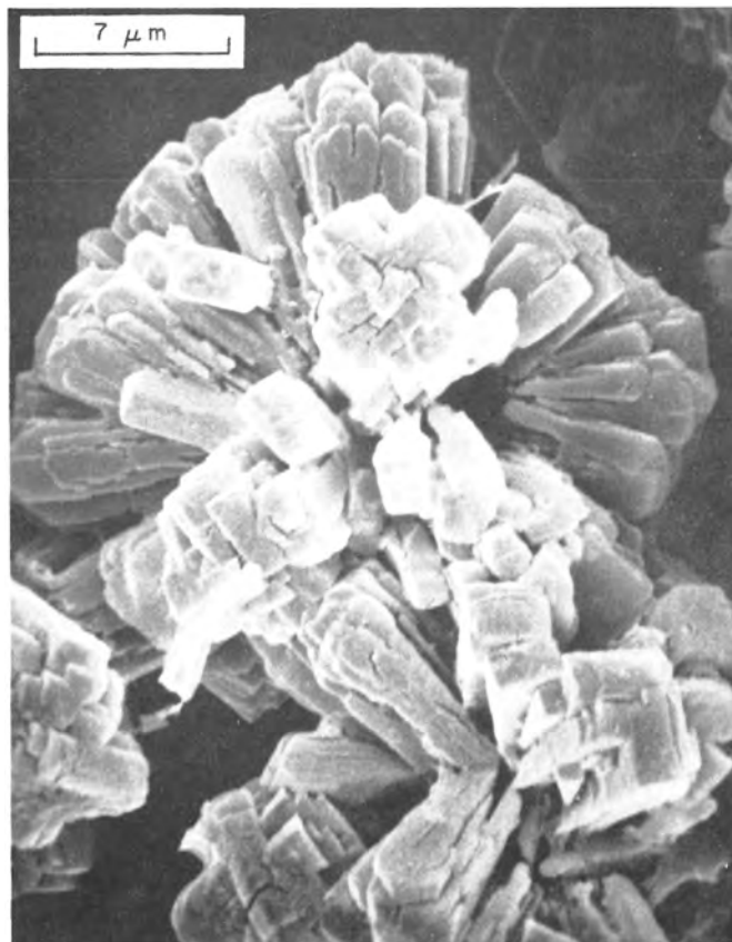
Figure 7-6.—Scanning electron micrograph of a phillipsite-rich tuff from a Pliocene lacustrine deposit near Durkee, Oregon, showing radial aggregates of prismatic phillipsite. Electron micrograph by M. J. Pinel, U. S. Geological Survey.
