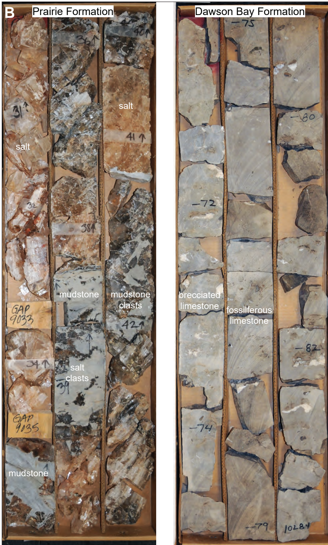
Figure 9B. Middle and early Late Devonian facies in core. The Prairie Formation (left) contains abundant salt deposits interbedded with intervals of mudstones. Photo from core W.H. Hass #1 (API#: 2509121328), Sheridan County, Montana. Core box height is 3 ft. Photo source: USGS, https://my.usgs.gov/crcwc/ . This example of mainly calcareous and dolomitic facies of the Dawson Bay Formation (right) is from Dawson County, Montana. Photo from core Burlington Northern 1 (API#: 2502121041), Dawson County, Montana. Core box height is 3 ft. Photo source: USGS, https://my.usgs.gov/crcwc/ .
