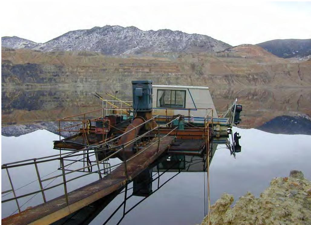
Figure 2-46d. MR pontoon boat is used for Berkeley Pit sampling. Boat is docked next to pump station used for pumping pit water to precipitation plant for copper recovery. (Photo courtesy of Daryl Reed, DEQ.)
