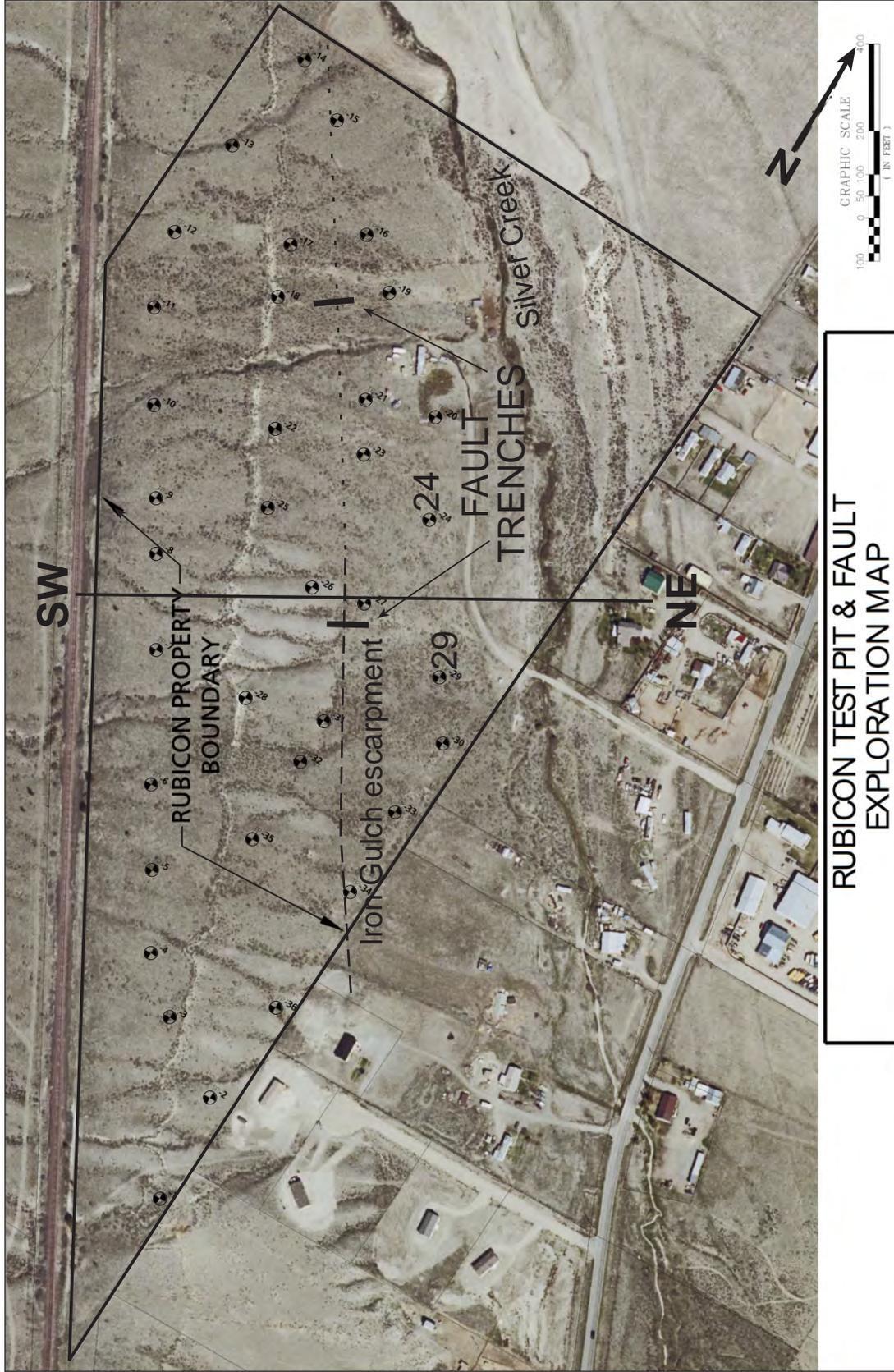
**Figure 3.** Map of the proposed development superimposed on a vertical aerial photograph showing the locations of soil test pits, trenches, the northern end of the Iron Gulch escarpment, and Silver Creek. The dotted northward projection of the escarpment indicates the Iron Gulch fault buried by young alluvial fan deposits by Stickney (1987). The line of section labeled SW-NE is shown in figure 12.
