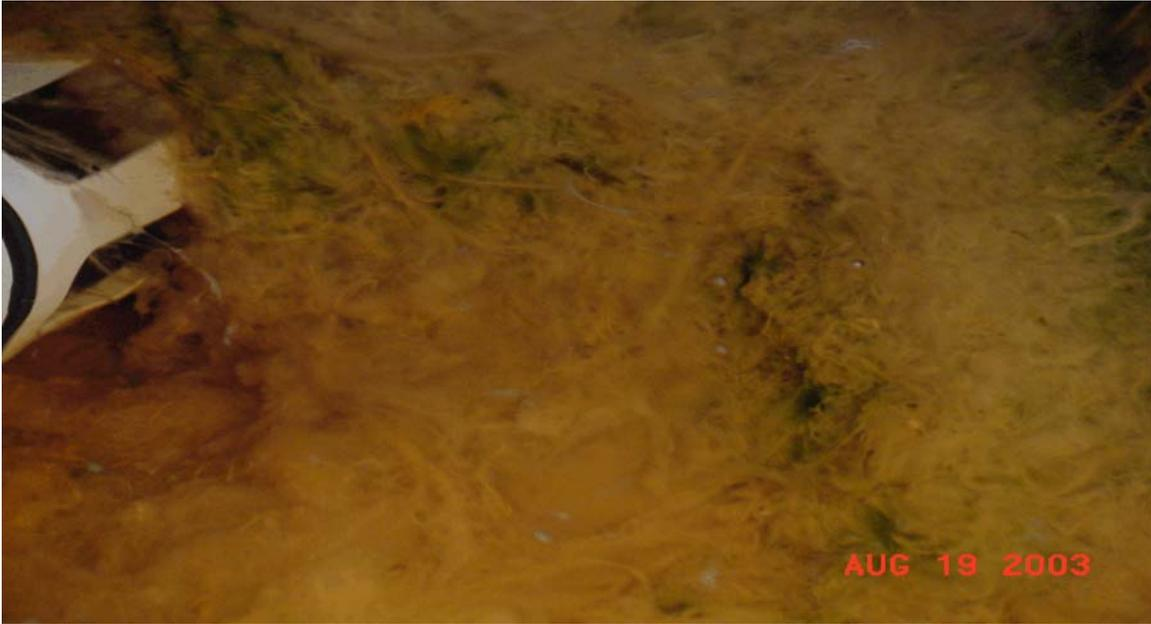
Figure 4.10 Photo of probe fouling by precipitates.
