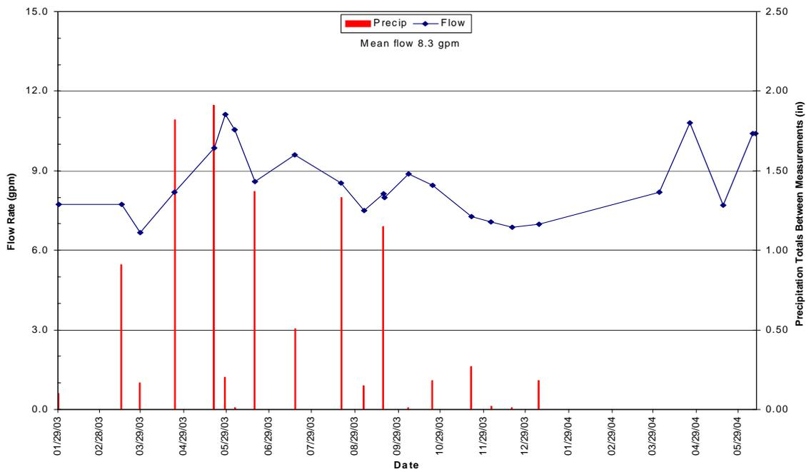
Figure 4.9 French Coulee drain hydrograph of measured flow rates with precipitation totals between measurements.
