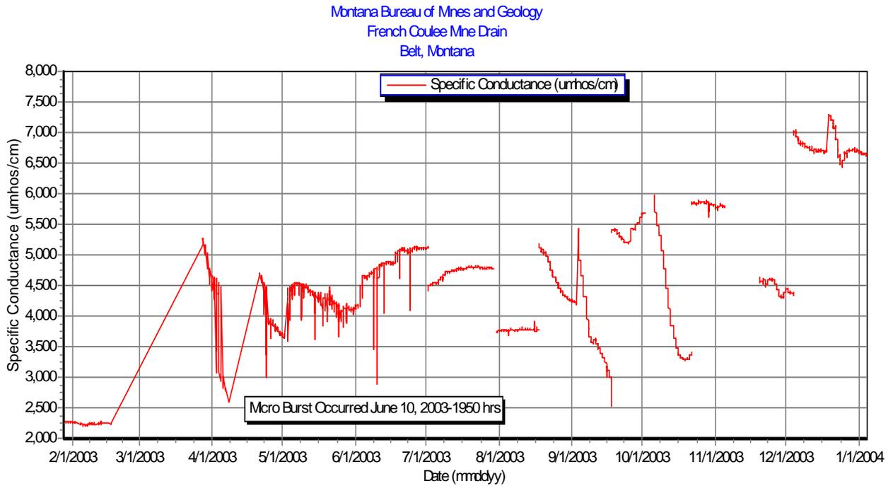
*Sonde relocated to drain pipe 6/4/03*
