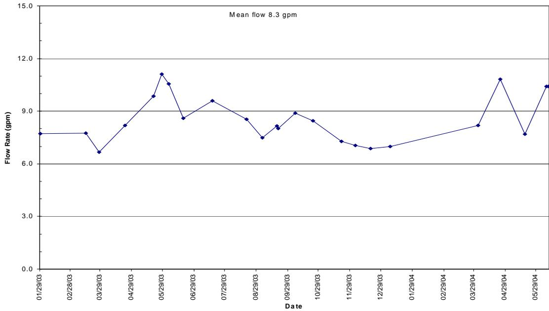
Figure 4.8 French Coulee Mine drain hydrograph of measured flow rates.
