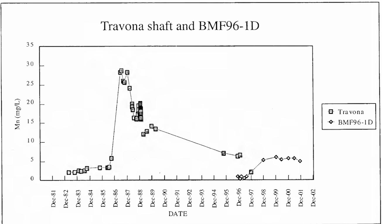
Figure 3-8. pH and manganese trends for the Travona Shaft and the replacement well, BMF96-1D
