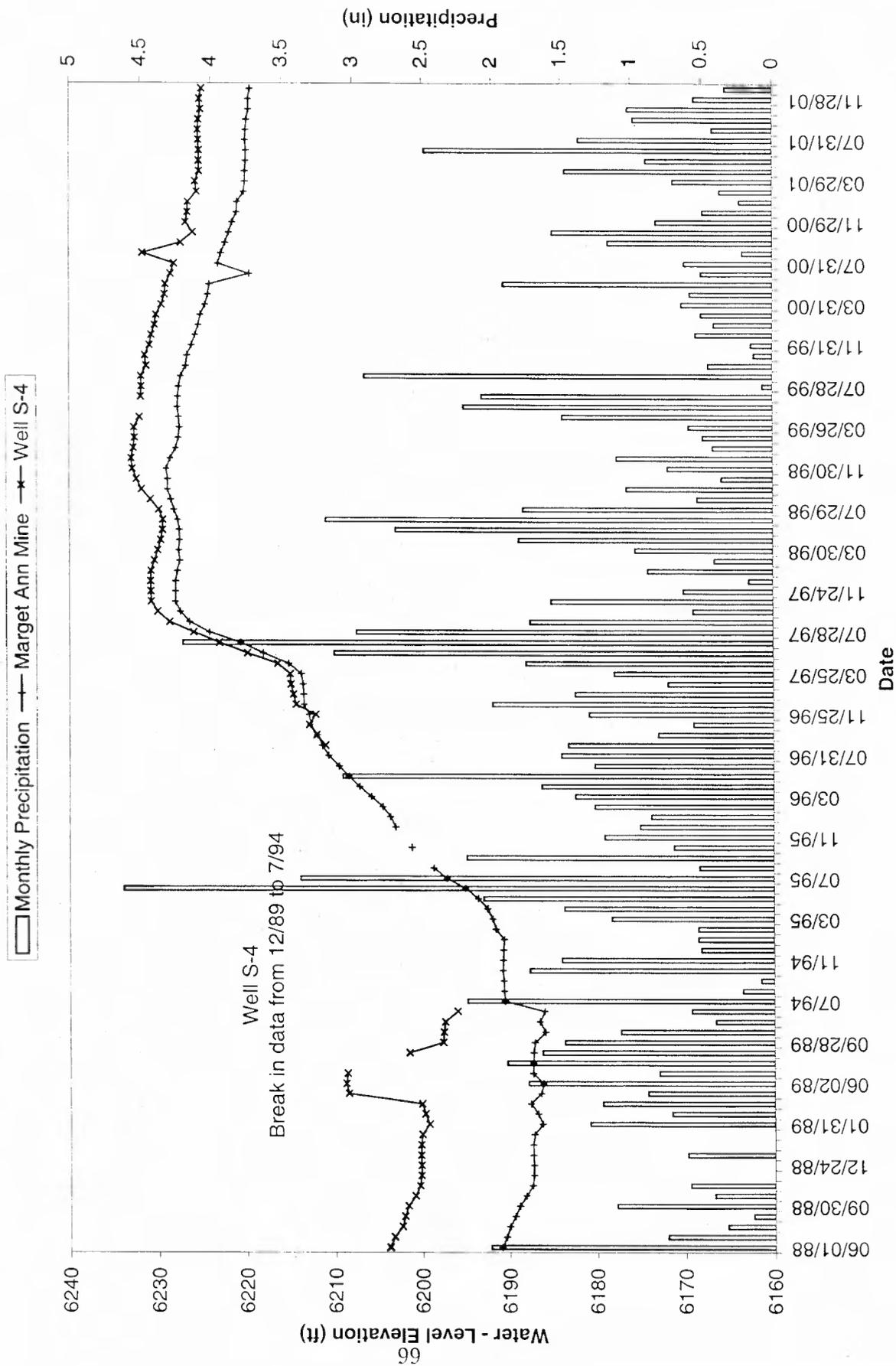
Figure 4-4. Water-level hydrographs for Marget Ann Mine and well S-4.
