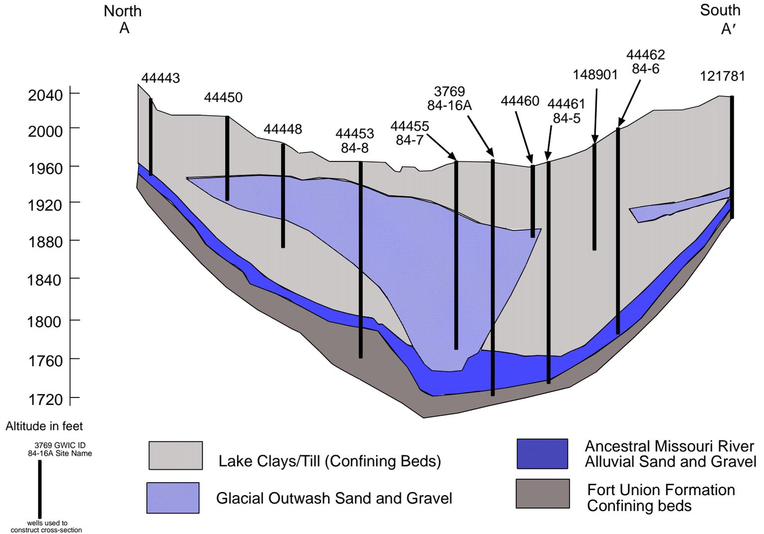
Figure 2. Geologic profile across the Clear Lake aquifer system east of Medicine Lake. See Figure 1 for location. Blue-colored units make up the Clear Lake aquifer system. Grey-colored units are aquitards.
