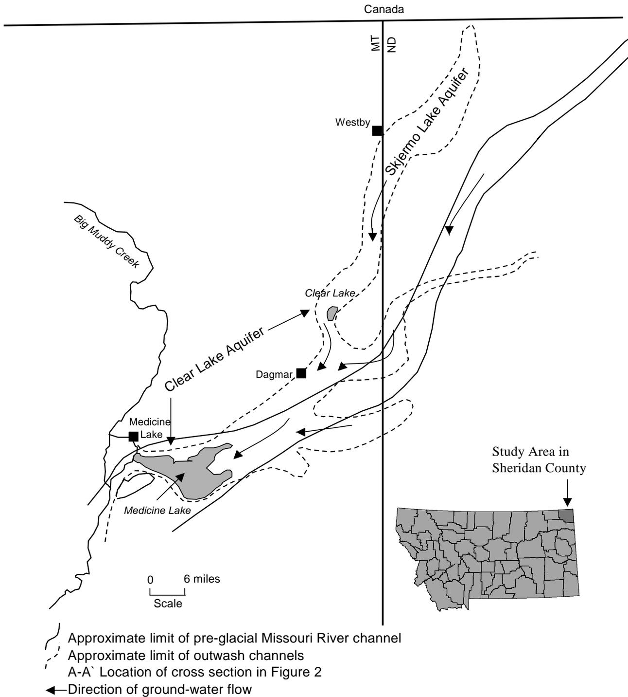
Figure 1. Buried pre-glacial channels of the Ancestral Missouri River and glacial outwash channels form the Clear Lake aquifer (MT). The Skjermo Lake aquifer is located within buried glacial outwash channels where they extend into North Dakota.
