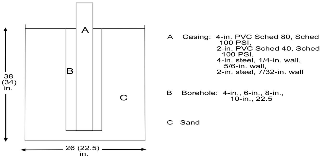
Figure 2. Schematic diagram of the laboratory calibration wells.
