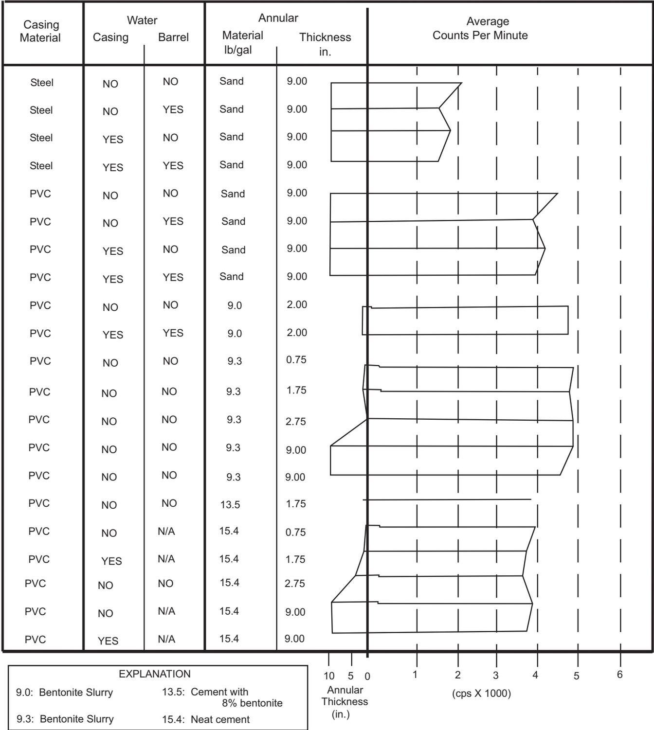
Figure 8. Tool response. Laboratory test: Gamma-gamma, focused, 100-mCi source, short spacing.
