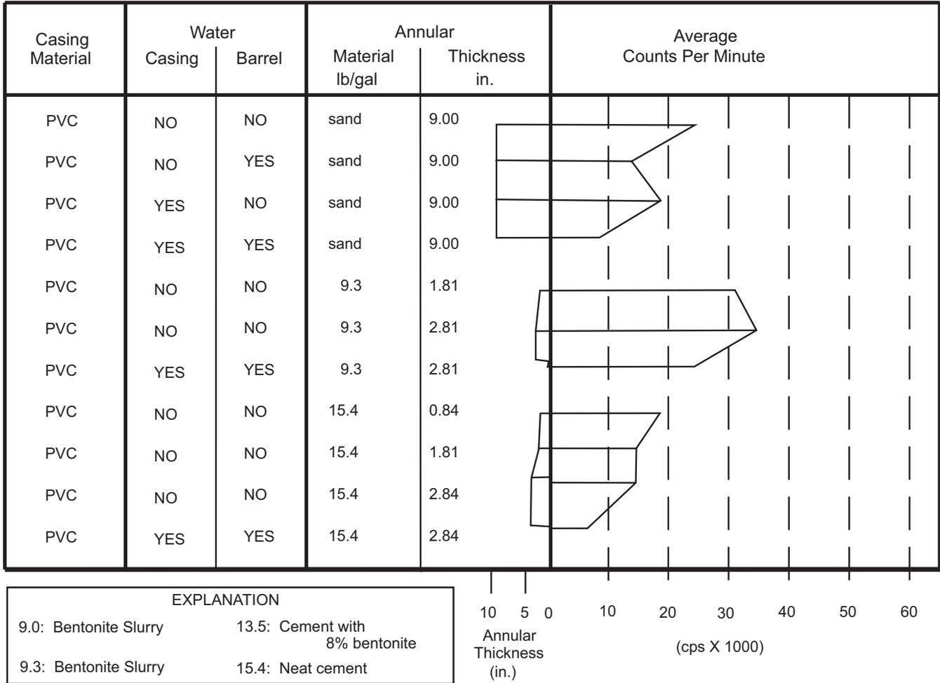
*Figure 6. Tool response, laboratory test: Gamma-gamma, 4pi, 18-in. spacing, 100-mCi source, 2-in. casing.*
