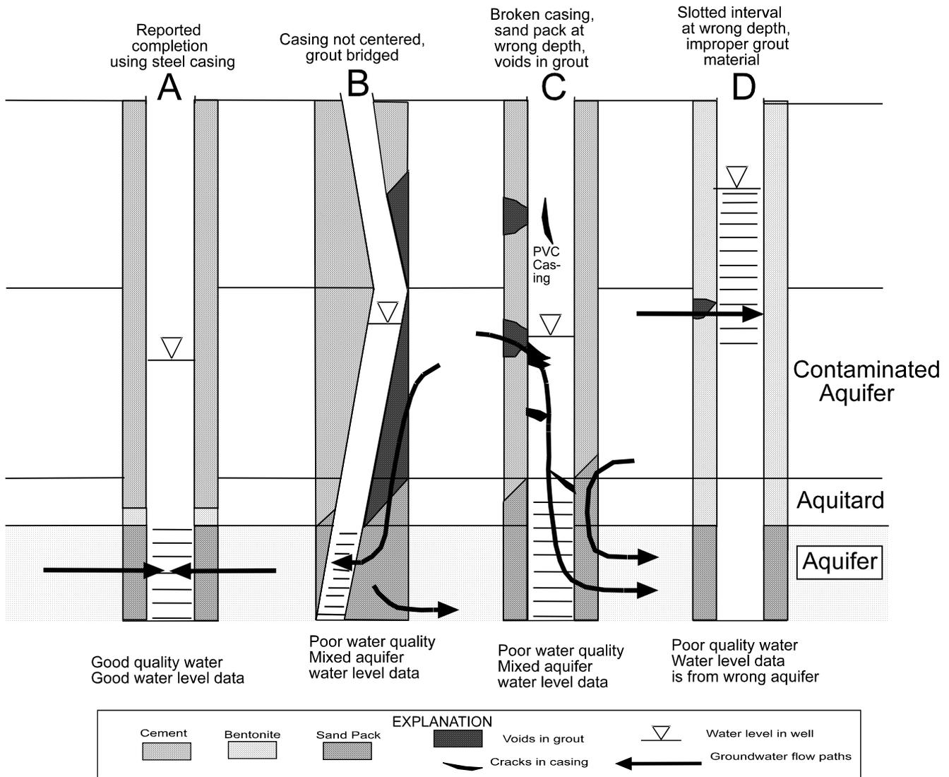
Figure 1. Examples of well completion problems.
