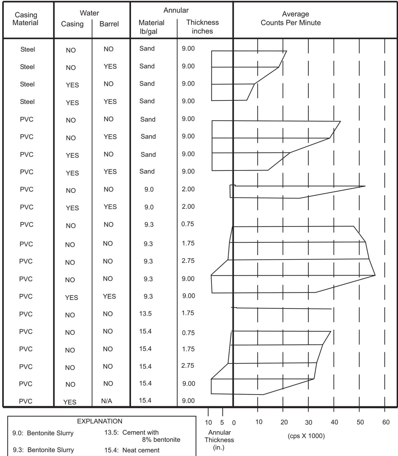
Figure 3. Tool response, laboratory test: Gamma-gamma, 4pi, 18-in. Spacing, 100-mCi source, 4-in. casing.1
