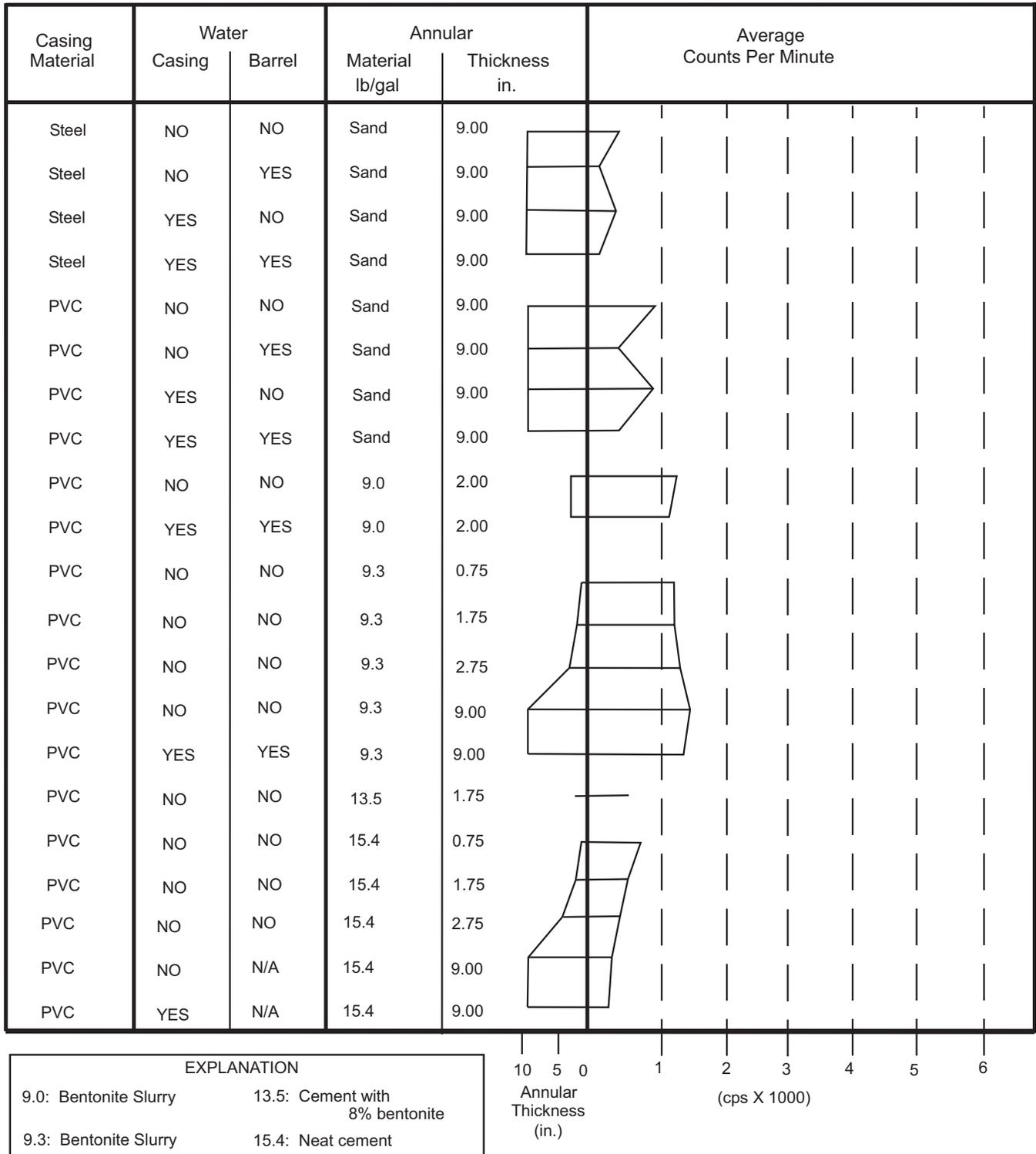
Figure 9. Tool response. Laboratory test: Gamma-gamma, focused, 100-mCi source, long spacing.
