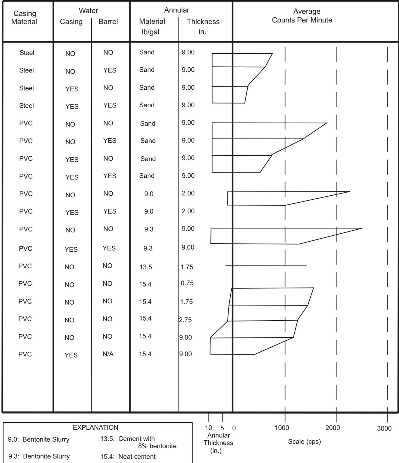
Figure 5. Tool response, laboratory test: Gamma-gamma, 4pi, 18-in. Spacing, 100-mCi source, 2-in. casing.
