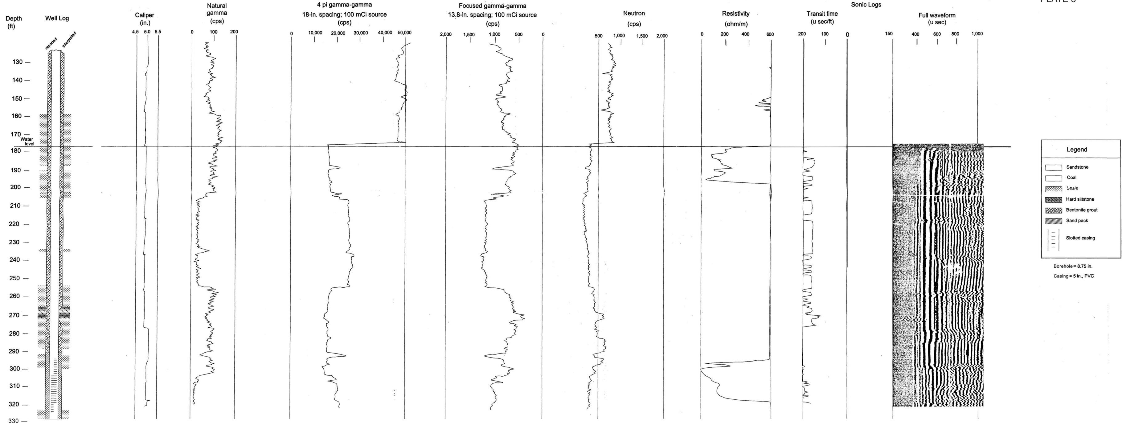
Plate 4. Well completion schematic and geophysical logs for well completed with PVC casing and cement grout.
