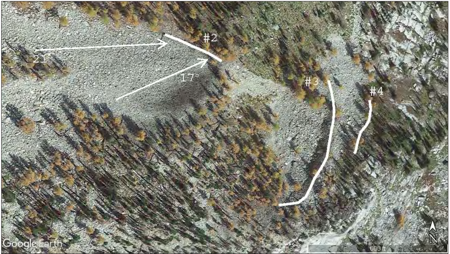
Figure 5. Thick white lines show locations of ramparts #2, #3, and #4 on a Google Earth image. Arrows show the orientations and slope angles of fall lines above rampart #2. Note that ramparts #3 and #4 are part of the same talus field, and could be interpreted as concentric flow features in a rock glacier.
