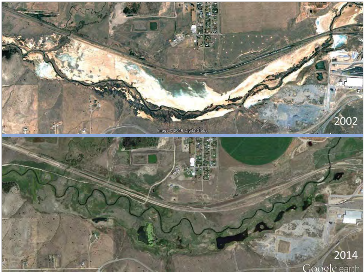
Figure 4. Before and after Google Earth images of SBC at Ramsay Flats. Whitish areas in 2002 photo are “slickens,” areas devoid of vegetation because of acidic soils with phytotoxic levels of metals. The small stream entering from the north, and west of small village of Ramsay, is Browns Gulch, one of two major tributaries to SBC.
