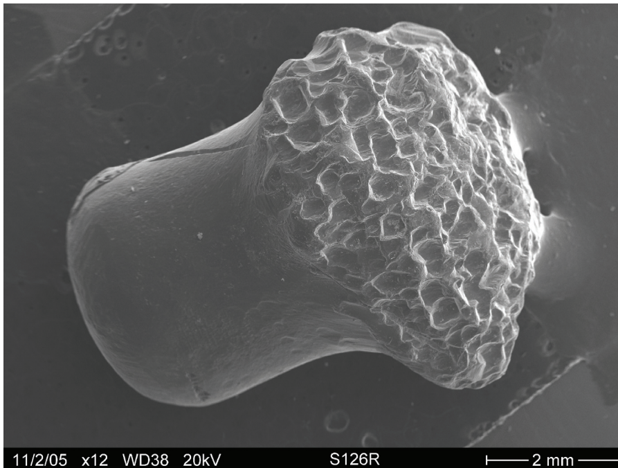
Figure 30. Scanning electron micrograph of sapphire from the South Fork of Dry Cottonwood Creek provided by Marc Bielenberg. Note grooves developed on smooth surface. See text for interpretation of surface features. Photo by Nancy Equall.
