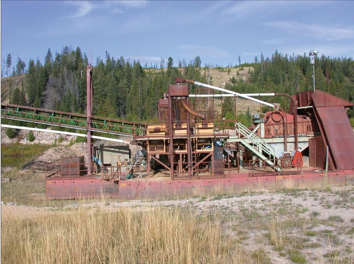
Figure 1.9. Floating washing plant in pond in 'the Meadow' constructed by Skalkaho Grazing, Inc.
