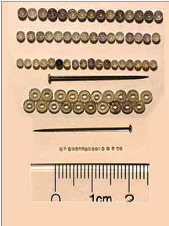
Figure 1.7. Watch or instrument bearings machined from sapphires mined from the Rock Creek sapphire district. Photo provided by Pete Antonioli.
