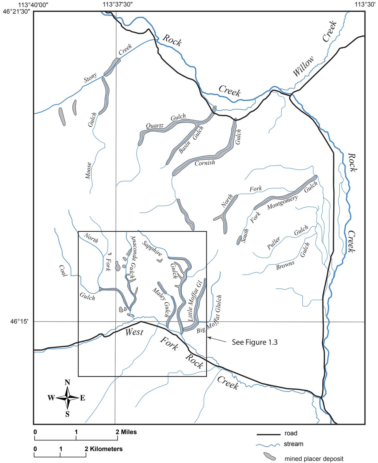
Figure 1.2. Gulches in the Rock Creek sapphire district from which sapphires have been recovered. With the exception of the southwestern part of the Rock Creek sapphire district, extent of placer mining from Robin McCulloch (oral commun., 2010.) See figure 1.3 for a more detailed map of the placer mining in the southwestern part of the Rock Creek sapphire district.
