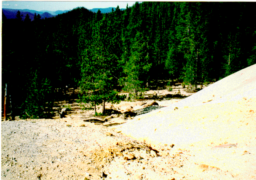
Figure 14B. Fined-grained material from the waste-rock dump has been washed several hundred feet downhill toward a small stream. The area was generally devoid of vegetation.
