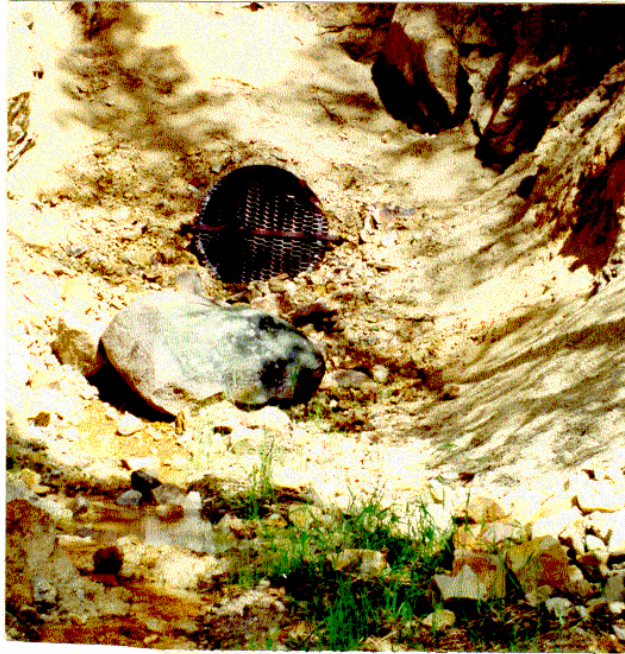
Figure 21A. The adit of the Cracker mine was open, but secure. A small discharge issued from the adit and flowed toward Cataract Creek. Ferric-hydroxide precipitate was evident along its entire length.
