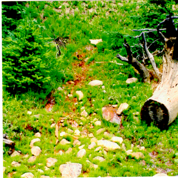
Figure 10A. There were at least two seeps at the base of the waste-rock dump. Ferric-hydroxide staining was evident in the seep closest to the dump.
