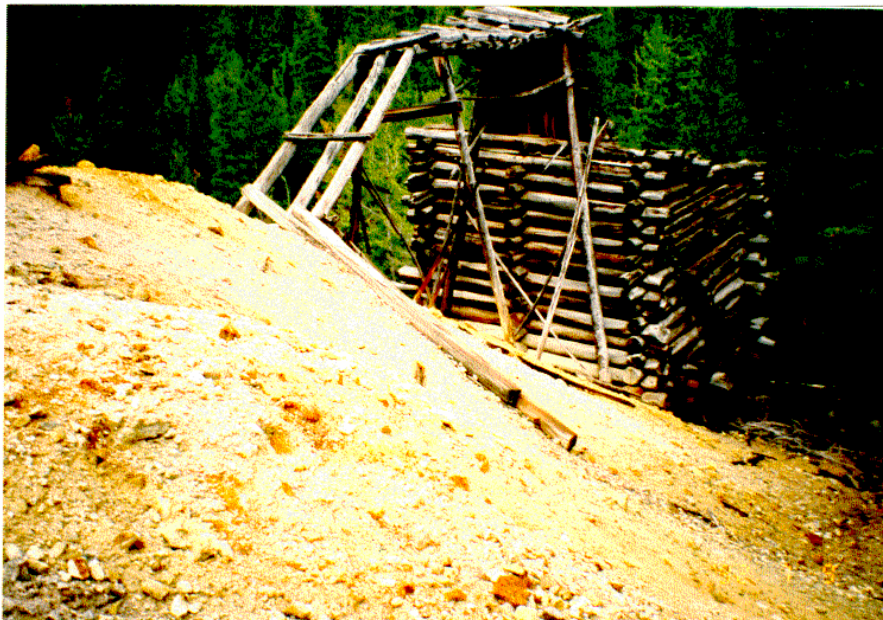
Figure 6B. Material from the waste-rock dump has been eroded and deposited on native soils below the dump. Some of this material is probably washed into the creek during runoff or precipitation.
