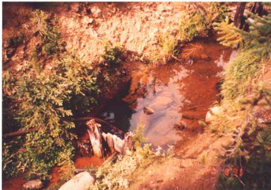
Figure 3.14 A ferric-hydroxide stained adit discharge (lower left) mixes with water flowing from flooded shaft S-1. The combined discharge flows into a wetland to the east.
