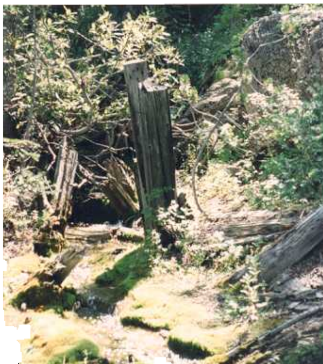
Figure 2.5 A small discharge issues from a collapsed adit at the Red Lion mine. The adit shown is on DNF administered land.
