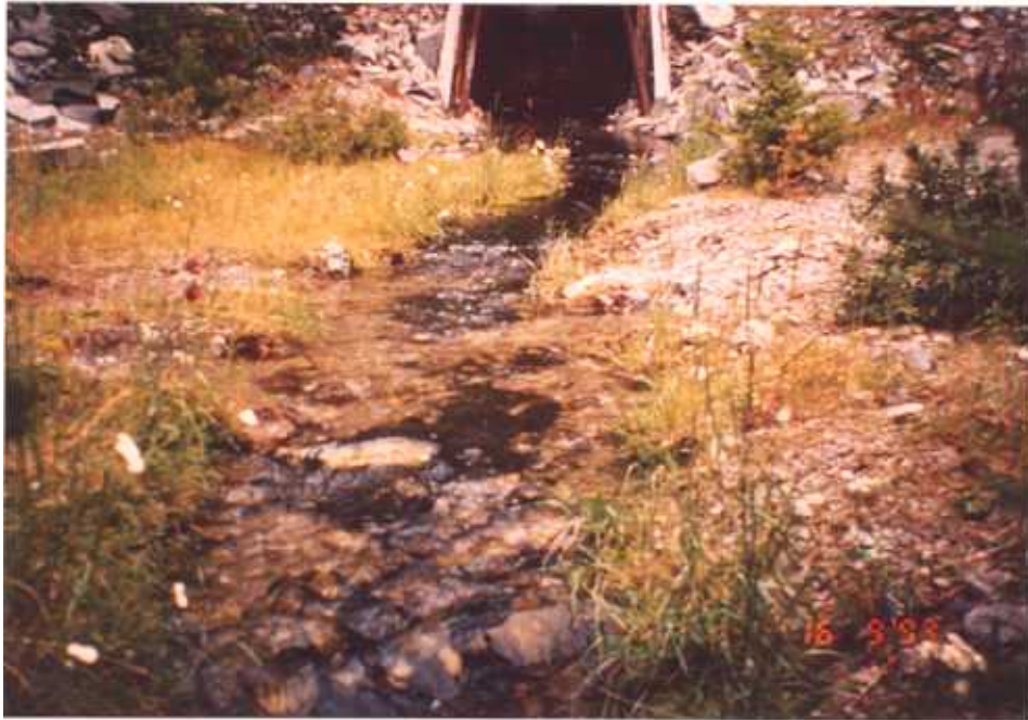
Figure 2.28 Water flowing from the adit crosses the top of the waste-rock dump.
