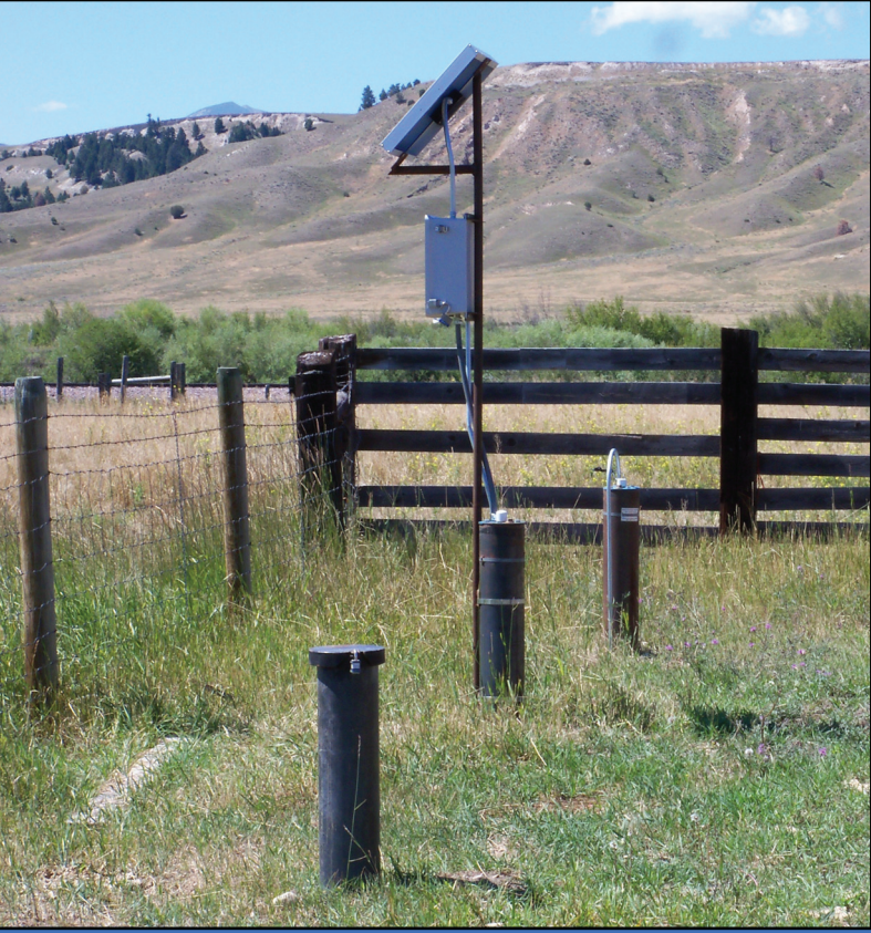
Nested monitoring wells in the Deer Lodge Valley with Tertiary sediments in the background. Photo by John LaFave, MBMG.
