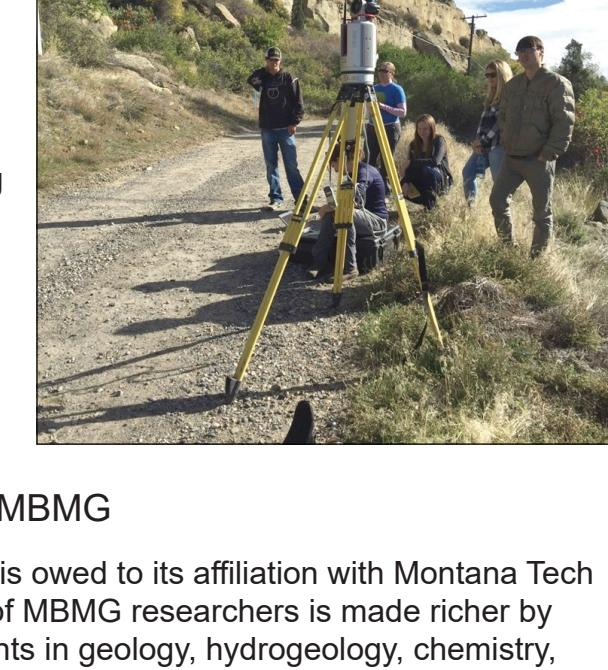
Figure 7. MBMG staff using LIDAR to compile detailed measurements of the Rimrocks in Billings.
