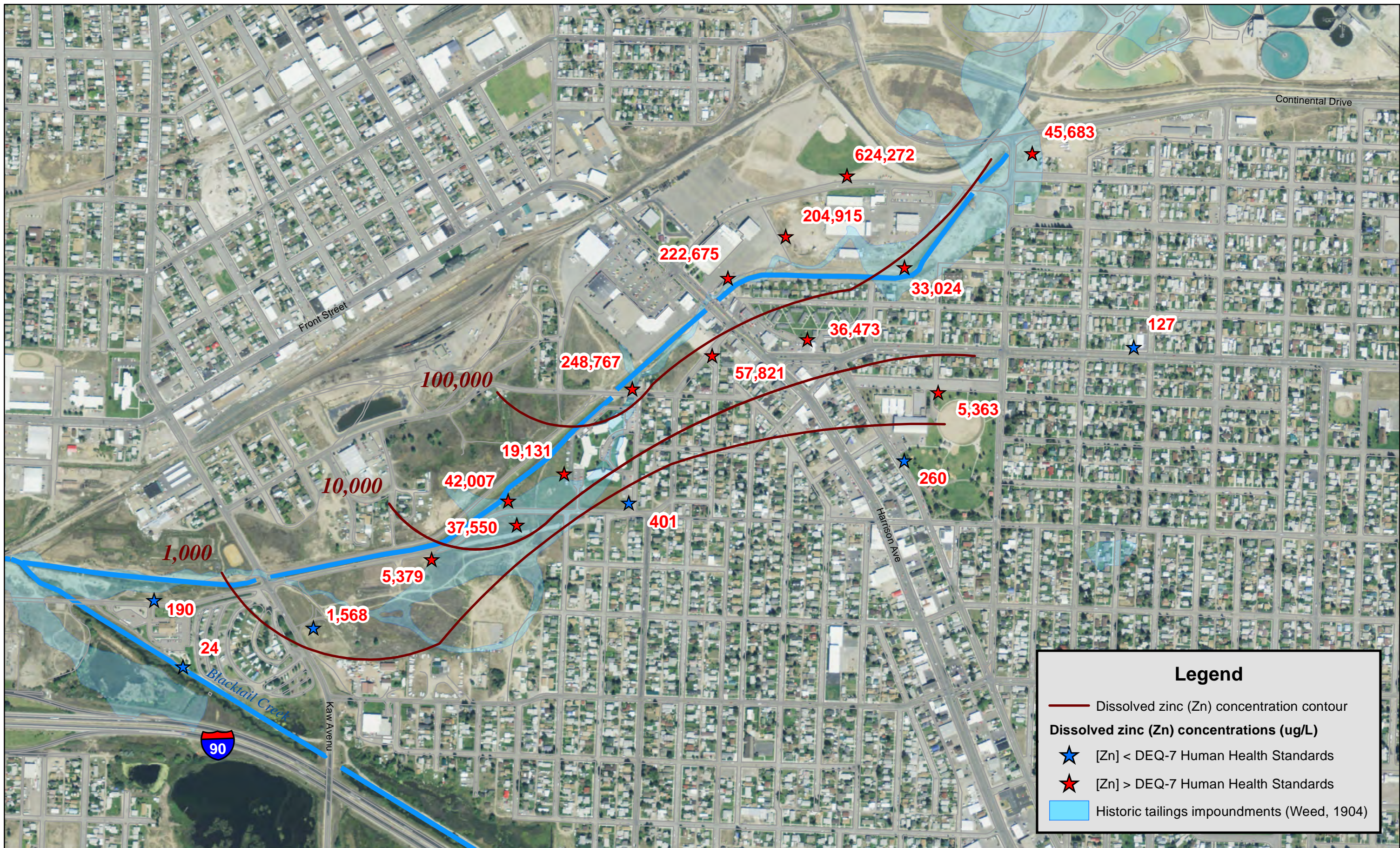
Figure 14. Dissolved zinc concentrations (ug/L) in the middle alluvial (MA) unit. Zinc contours are on a log scale.
