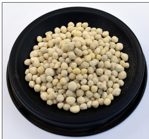
Figure 2. A sample of small diammonium phosphate granules. These water-soluble granules are used as fertilizer to add P and nitrogen to soil depleted by extensive cultivation. Photo by Suyash Dwivedi (CC-BY-SA-4.0)
