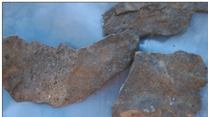
Figure 3. A sample of phosphorite with 32 wt.% P_2O_5 and ~0.3 wt.% REEs from Granite County, Montana. Photo by Adrian Van Rythoven (MBMG).
