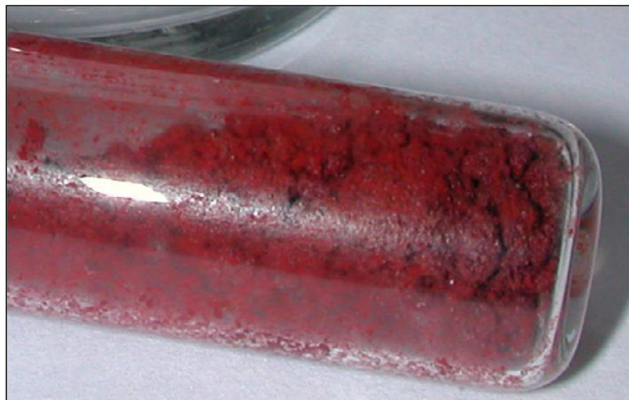
Figure 1. A vial of red P, one of the four varieties of elemental P. Red P is used for safety matches. Photo by Tomihahndorf (public domain).
