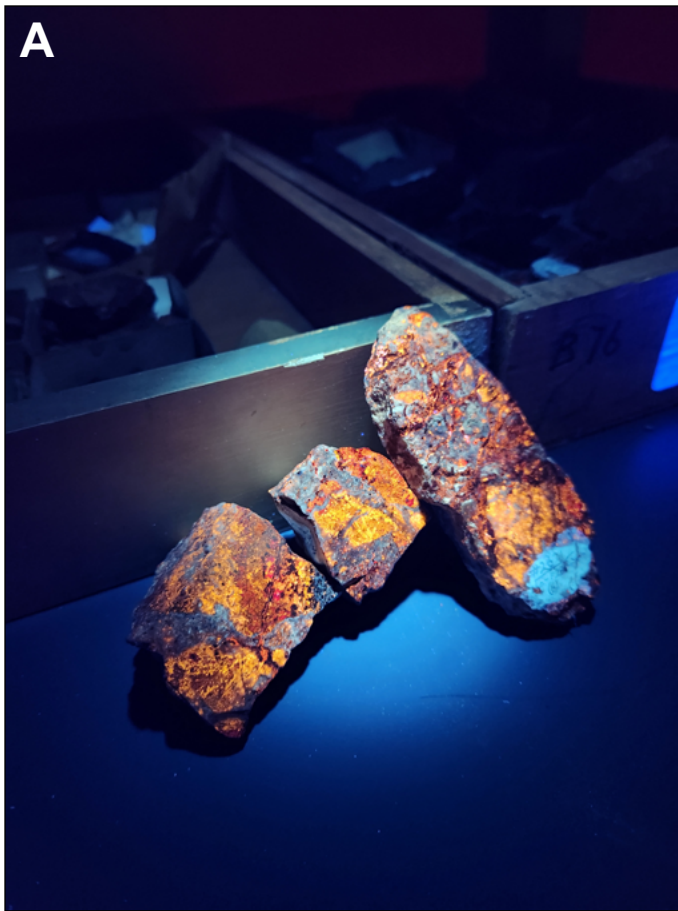
Figure 3. UV-fluorescent sphalerite from the Anaconda Research Collection. Fluorescence of sphalerite is related to trace element content and can indicate important byproduct critical commodities. (A) UV-fluorescent sphalerite from the Leonard Mine, Butte District. (B) UV-fluorescent sphalerite from the Badger Mine, Butte District.
