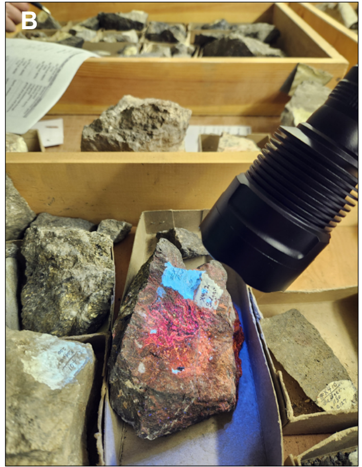
Figure 3. UV-fluorescent sphalerite from the Anaconda Research Collection. Fluorescence of sphalerite is related to trace element content and can indicate important byproduct critical commodities. (A) UV-fluorescent sphalerite from the Leonard Mine, Butte District. (B) UV-fluorescent sphalerite from the Badger Mine, Butte District.
