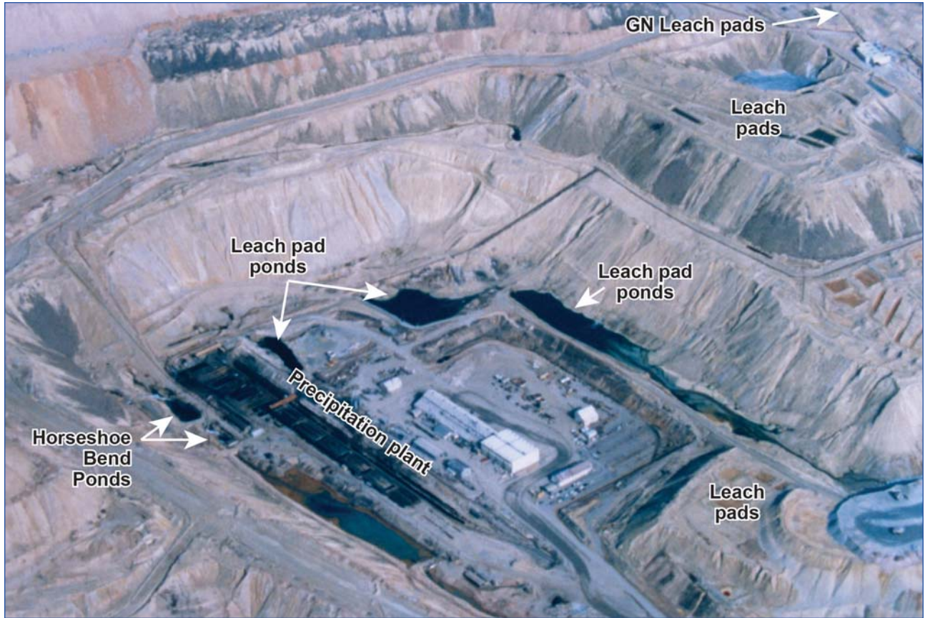
Figure 10. Location of leach pads, leach circuit ponds, and Horseshoe Bend ponds (1998). View is from southwest looking northeast.
