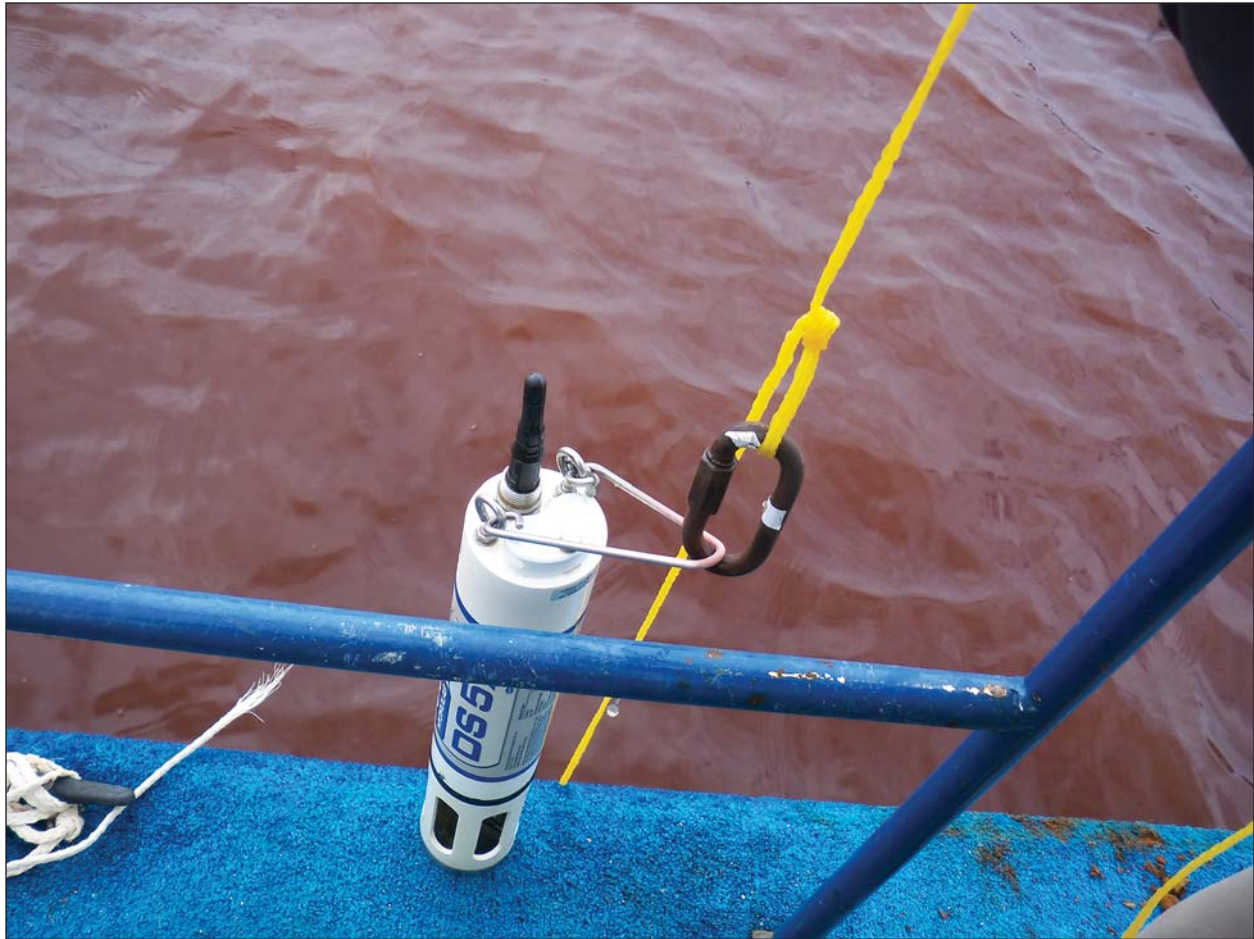
Figure 37. Photo of Hydrolab DataSonde Model DS5x used for Berkeley Pit profiling.
