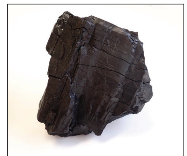
Figure 4. A subbituminous coal sample approximately 5" x 5" from the Dietz Bed of the Spring Creek Mine, Big Horn County, Montana. Photo by Ryan Davison, MBMG.
