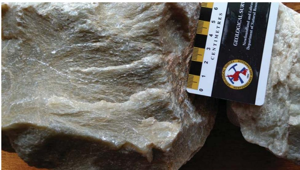
Figure 4. Typical samples of high-grade Montana talc. Massive block on the left and sheared and foliated talc on the right. Shear foliation and rehealed breccia zone in sample on the right is at approximately a 20° angle to the long axis of the scale card.
